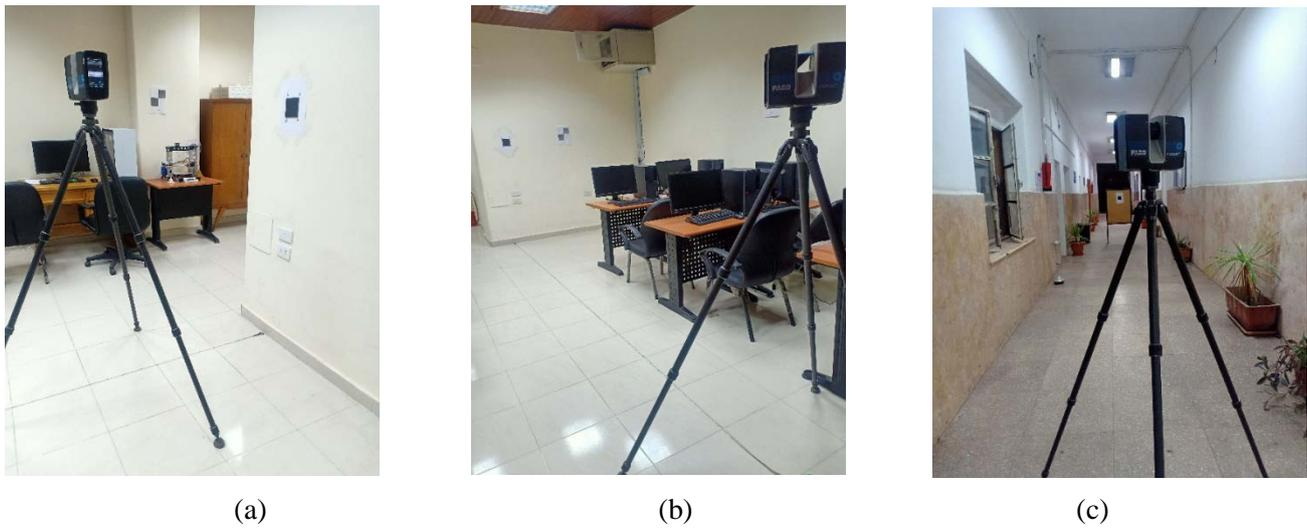
**Figure 3:** Scanner positions for three cases studied (a- at 1 m, b- at 5 m and c- at 10 m, respectively).
