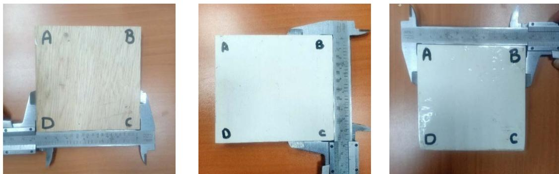
**Figure 4:** Measuring the dimensions of each block using the vernier.
