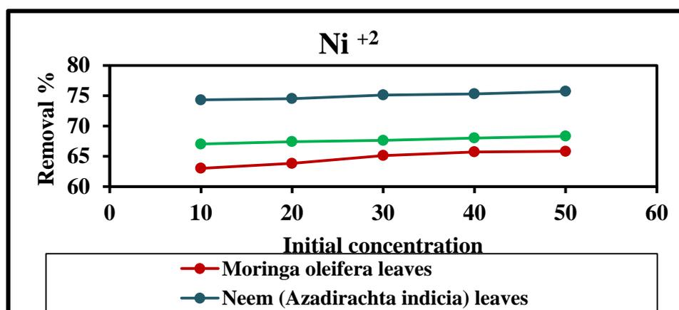
**Fig. (2)** Removal percentage of  $\text{Ni}^{+2}$  using ZnO-NPs from different green leaves.
