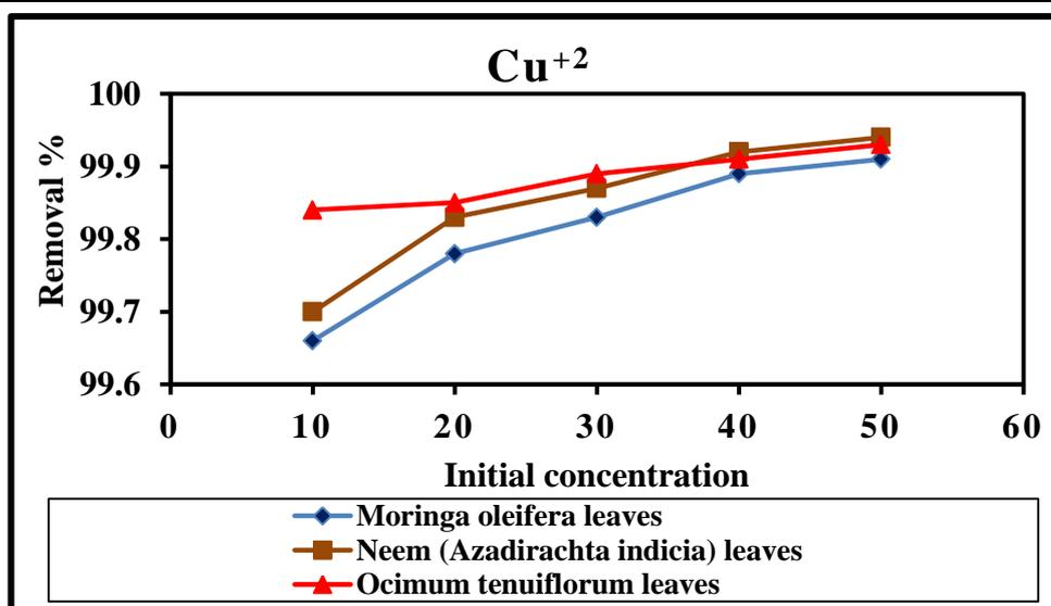
**Fig. (1)** Removal percentage of  $\text{Cu}^{+2}$  using ZnO-NPs from different green leaves.
