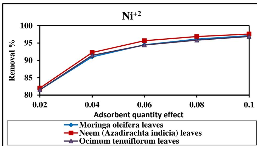
Fig. (4) Removal percentage of  $Ni^{+2}$  using ZnO-NPs from different green leaves
