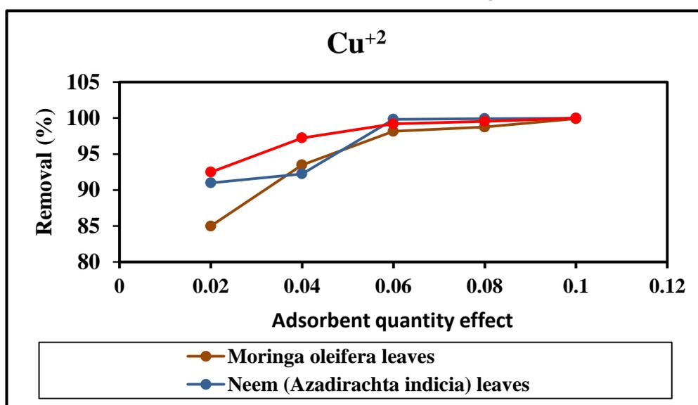
Fig. (3) Removal percentage of  $Cu^{+2}$  using ZnO-NPs from different green leaves.
