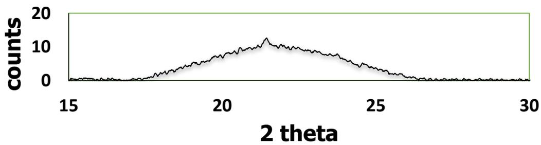
Fig. (3) XRD pattern of Nano K- Silicate
