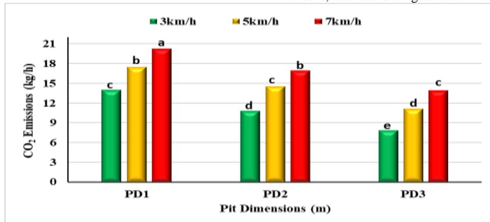
Fig. (23) Environmental impacts of study treatments on CO<sub>2</sub> emissions (t). Values followed by different letters are significant at  $p < 0.05$  and L.S.D = 1.7789.
