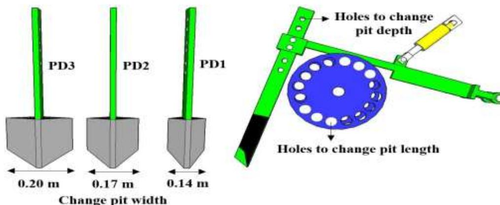
Fig. (9) Mechanism of changing the dimensions of pits.
