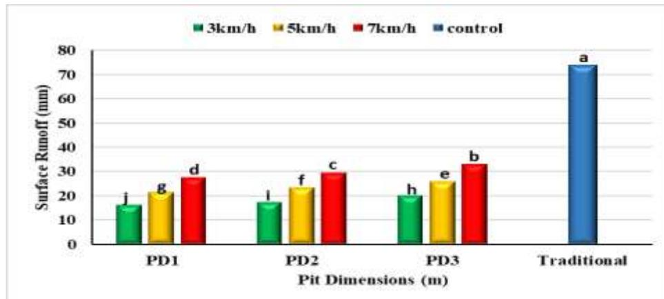
Fig. (18) Influence of treatments on rainwater runoff (mm). Values followed by different letters are significant at  $p < 0.05$  and L.S.D = 0.7839.
