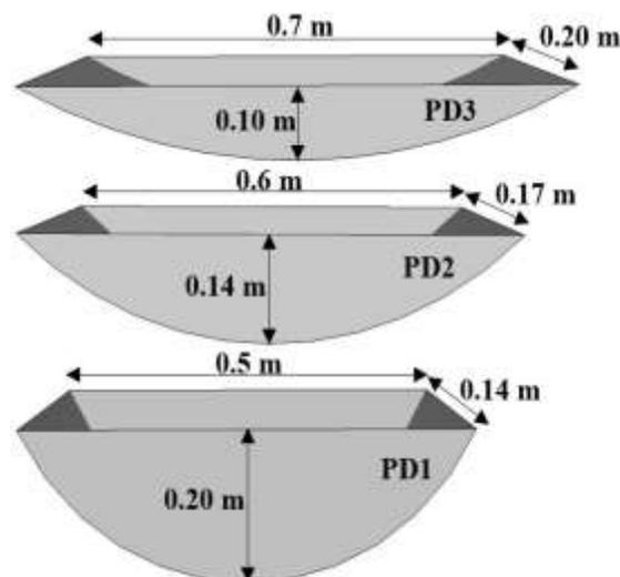
**Fig. (6)** Illustration of the dimensions of rainwater harvesting pits.
