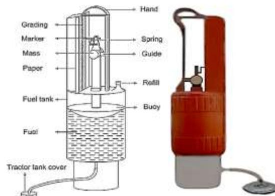
Fig. (4) Fuel meter for measuring fuel consumption [11].
