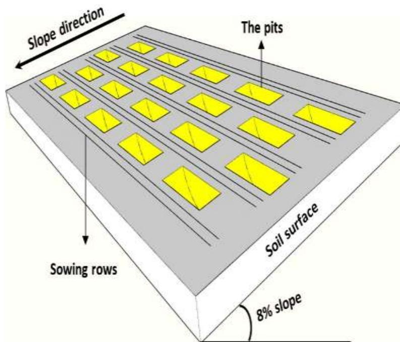
**Fig. (7)** Illustration of length of pits perpendicular on slope direction.
