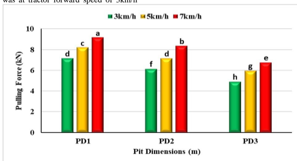
**Fig. (15)** Influence of treatments on pulling force (kN). Values followed by different letters are significant at  $p < 0.05$  and L.S.D = 0.1193.
