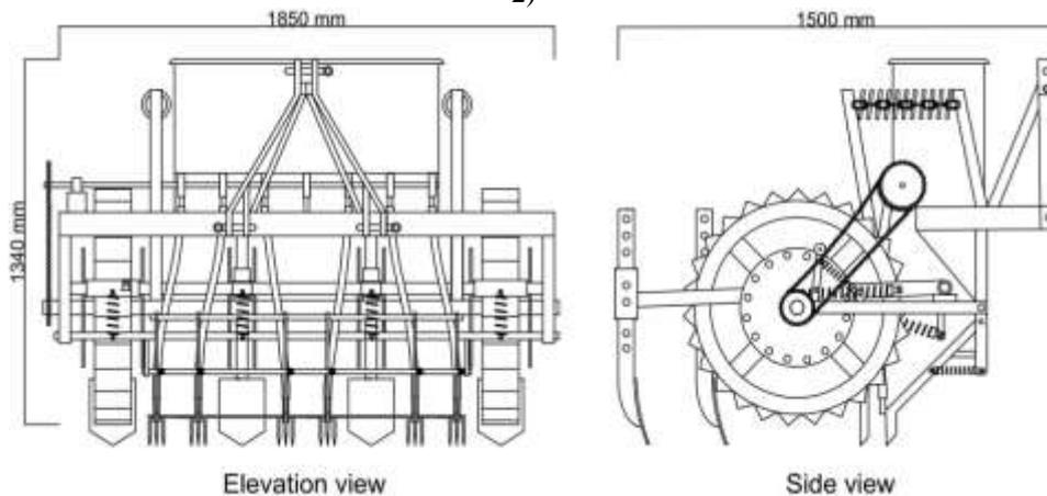
Fig. (2) Elevation and side view for study machine.
