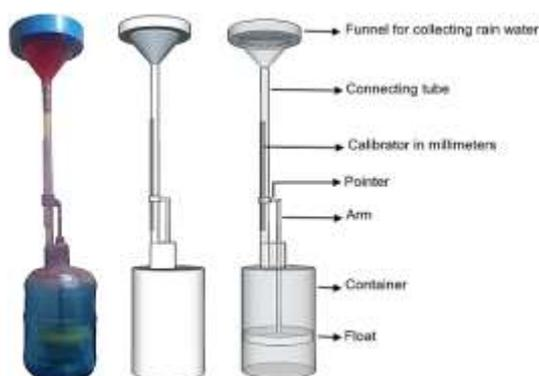
Fig. (3) Rain gauge device for measuring rainwater falling in the field [1].
