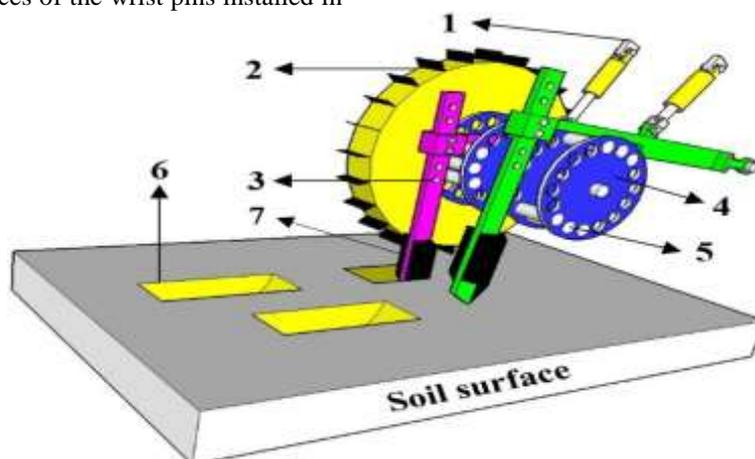
Fig. (8) The mechanism of making pits by the study machine.
