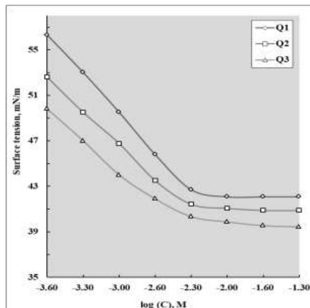
**Figure 3: Surface tension-log concentration of the prepared diquatery derivatives (Q1-3) at 25 °C.**
