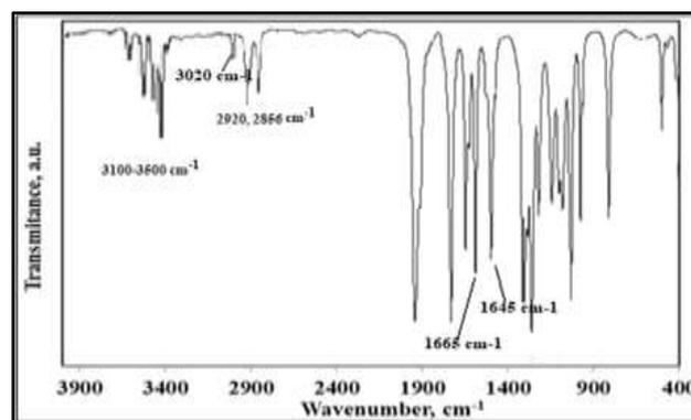
Figure 2: FTIR spectra of diquaternary (Q1).
