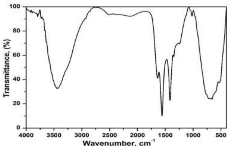
Fig. (1) FTIR of  $ZrO_2$  nanoparticles (ZU sample) using auto-combustion method and urea as a fuel.
