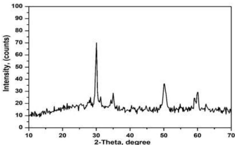
Fig. (2) XRD of  $ZrO_2$  nanoparticles (ZU sample) using auto-combustion method and urea as a fuel.
