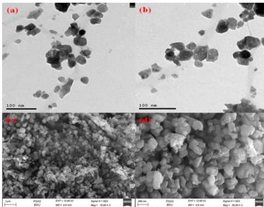
**Fig. (3)** HR-TEM (a and b) and FE-SEM (c and d) of zirconium oxide nanoparticles (ZU sample).
