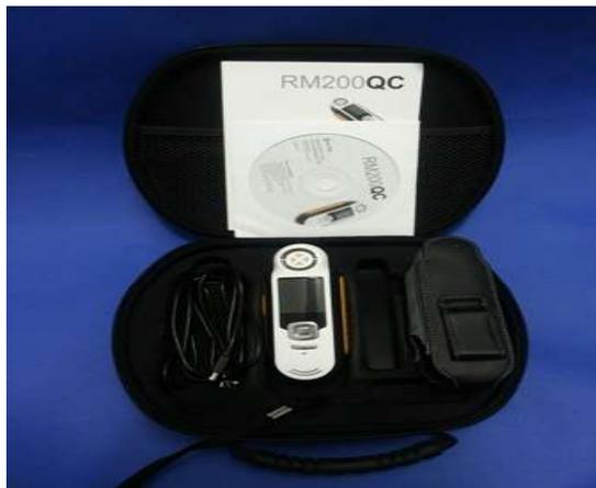
**Figure 2:** Portable Reflective Spectrophotometer
