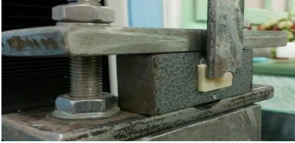
**Figure 1:** Mounted samples on a computer controlled Universal testing machine.
