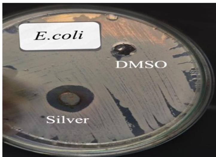
Figure 4. Displays the inhibition zone diameter that resulted from the anti-bacterial action of silver nanoparticles against *E.coli*. Dimethyl sulfoxide has been used as a control.
