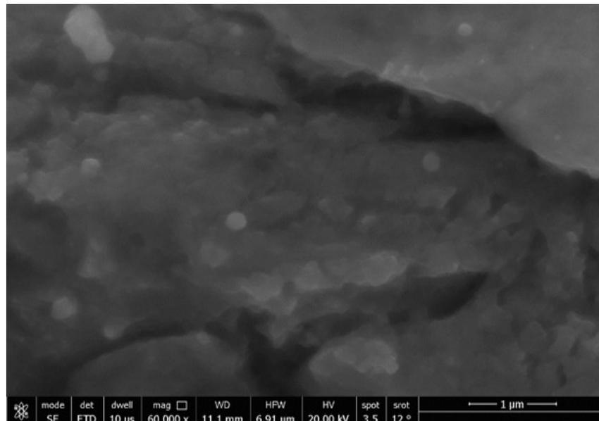
Figure 3. demonstrates the SEM image of silver nanoparticles
