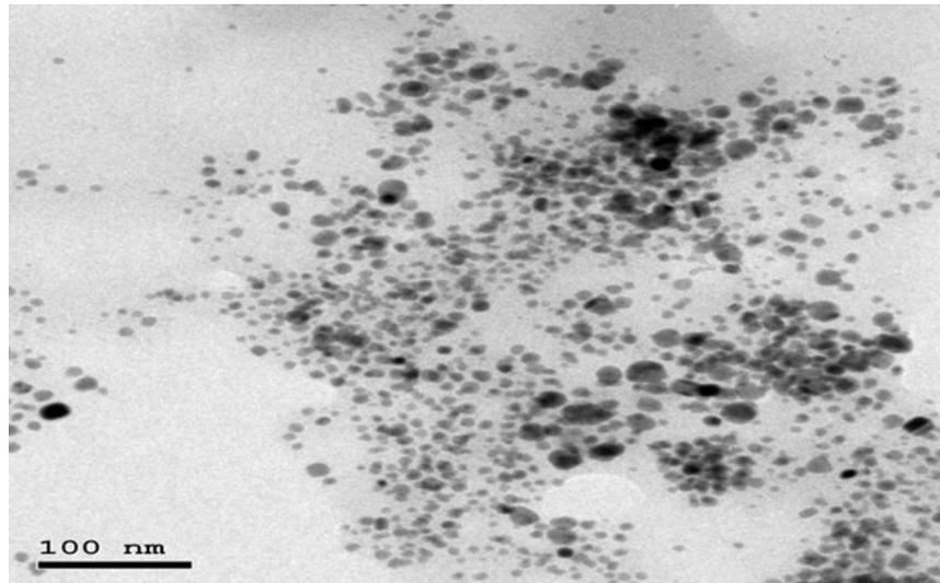
Figure 2. shows TEM image of silver nanoparticles which revealed the average size of silver nanoparticles.
