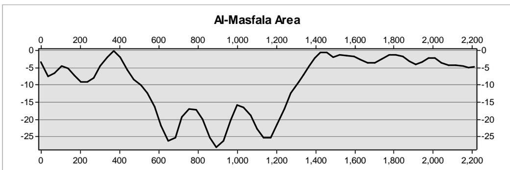
Figure (17): A cross section on the road axis showing the depth of the water.
