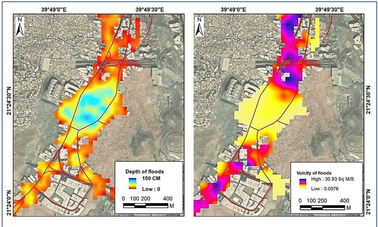
Figure (15): Hydraulic simulation for automatic identification of buildings and roads exposed to the risk of flash floods in the Al-Masfala area, south of the Holy Mosque of Mecca.
