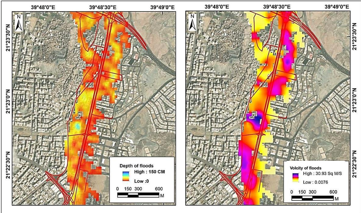
**Figure (23):** Hydraulic simulation for automatic identification of buildings and roads at risk using the Batha Quraish diagram.
