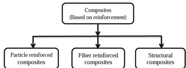
**Fig. 1** composites types according to kind of reinforcement [18].
