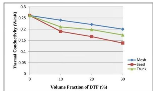
**Fig.5.** DPF/ epoxy composite thermal conductivity with the fiber content [97].
