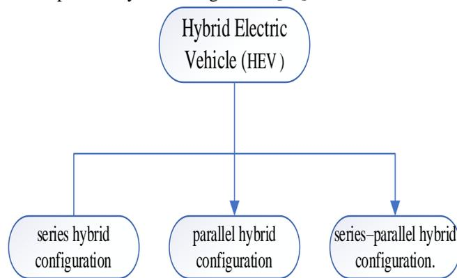
**Fig. 1:** Classification based upon the structure of HEV.
