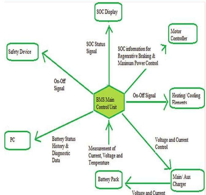
**Fig. 3:** Functions of battery management system.
