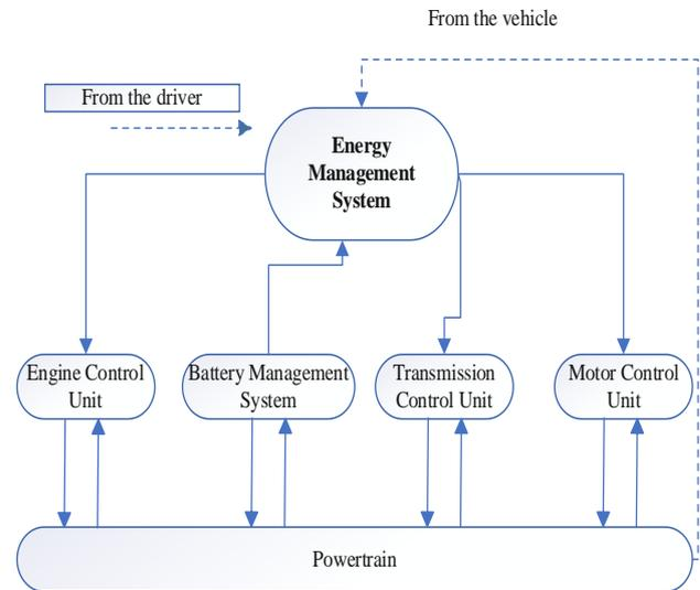
**Fig. 4:** control scheme of an HEV.
