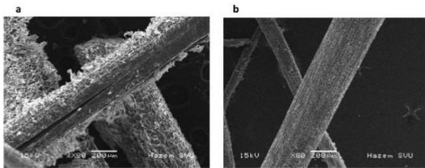
**Fig. 3** SEM of (a) Untreated date palm fiber and (b) Treated date palm fiber with 5 % NaOH [54]
