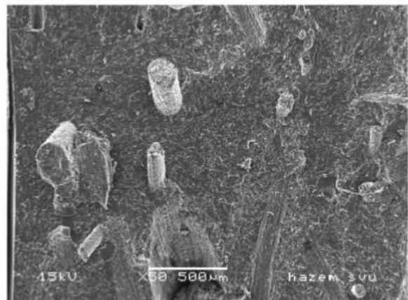
**Fig .4** SEM micrograph of fracture surface of date palm fibre/polyester composite[54]
