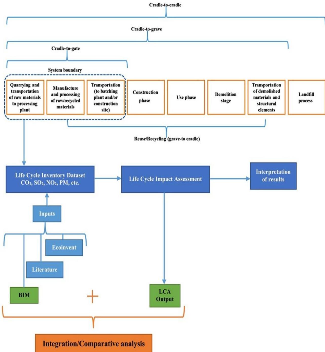
Fig. 3 System boundary of LCA application in this article
