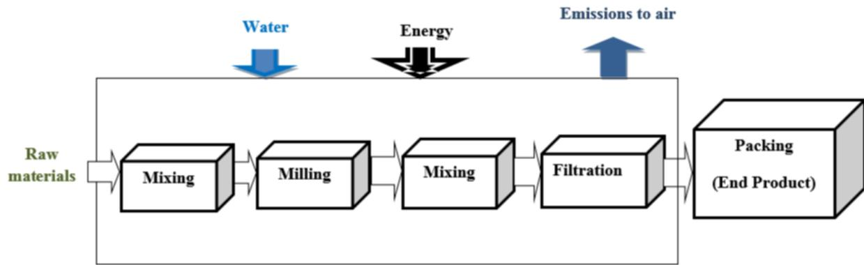
Fig. 4 System boundary of the paint production [16]
