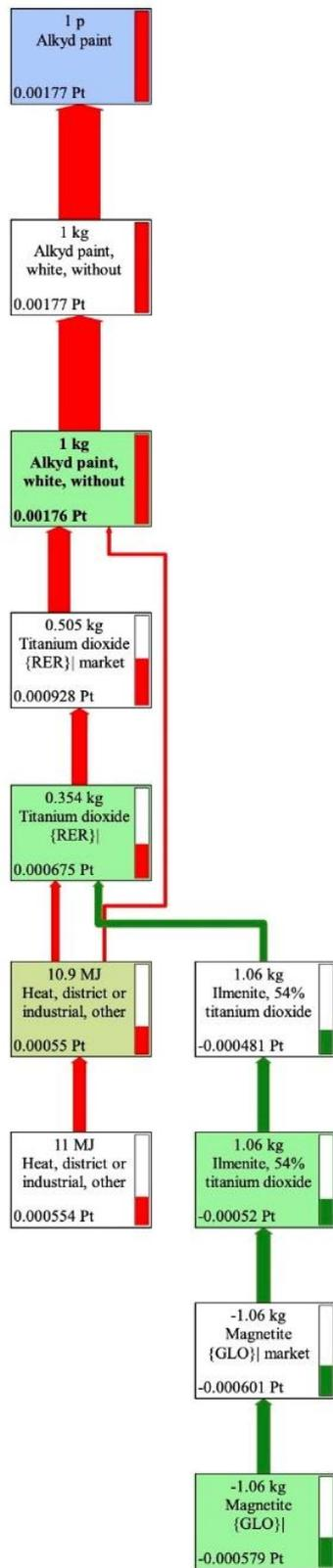
Fig.6 (a) Network flow of Alkyd Paint
