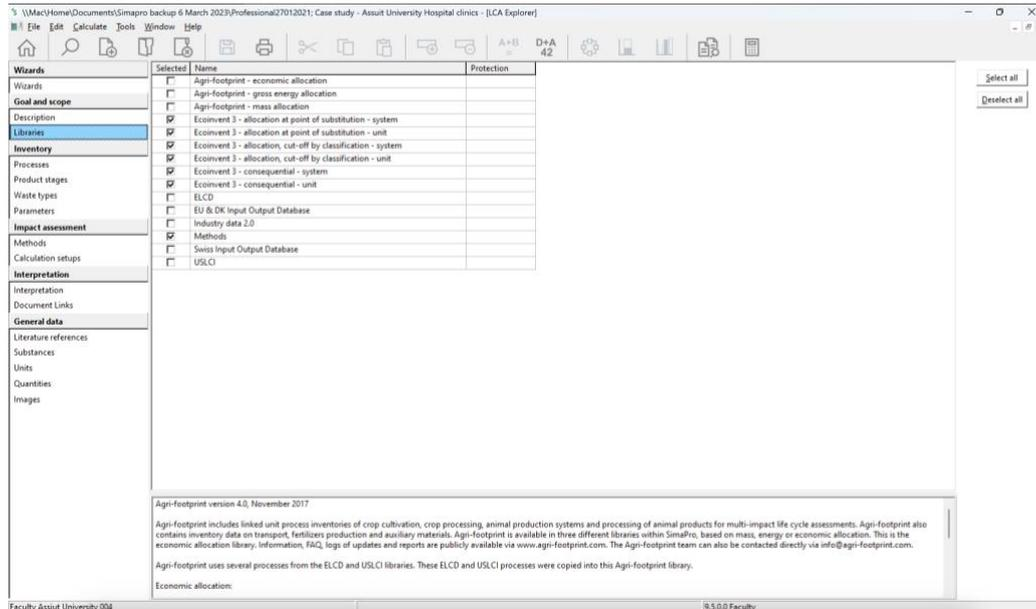
Fig. 7 Ecoinvent database embedded in SimaPro V9.5
