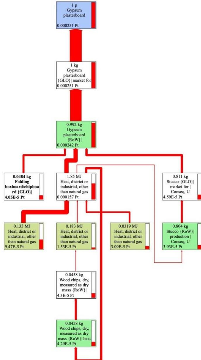
Fig.6 (b) Network flow of Gypsum Plasterboard
