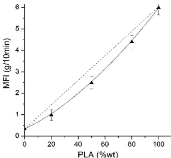
**Fig. 6** Melt Flow Indices (MFI) were determined following ISO 1133 using a CEASt modular
