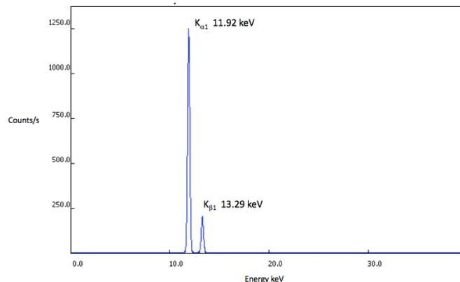
**Fig. 7** XRF spectrum of bromine
