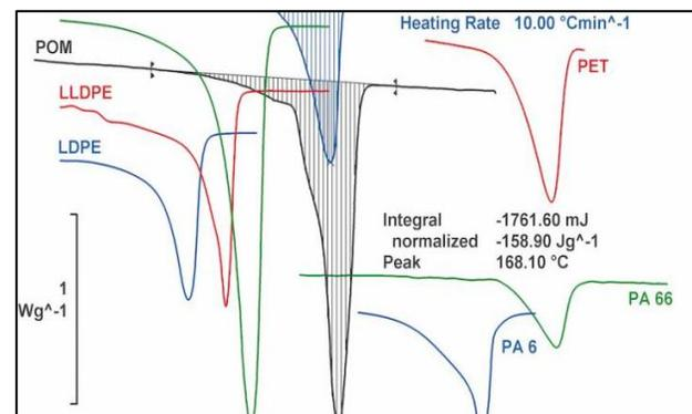
Figure 3 Mettler Toledo DSC 821
