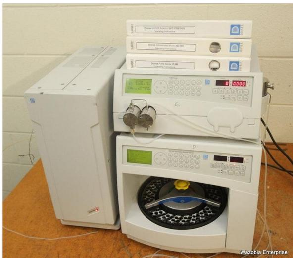
**Fig. 5** Dionex ASI-100 automated sample injector, a Gynkotex Model 300 high-precision pump, an Erma ERC3612 degasser, and a Spark Holland Mistral column oven.
