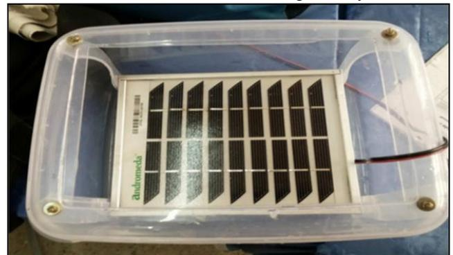
**Fig. 4** Liquid immersion cooling of PV panels [14].
