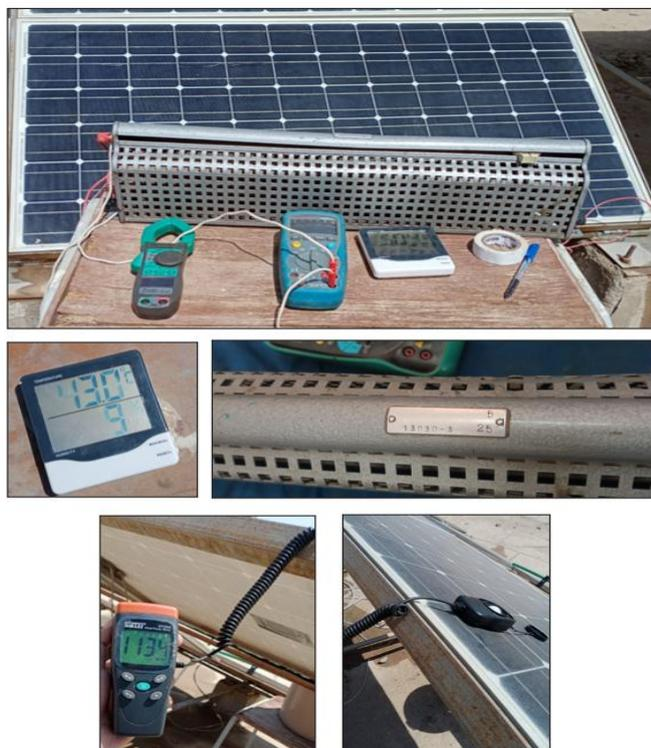
**Fig. 12** Tools used for measuring panel voltage, current, temperature and radiation of PV panels; Renewable Energy Laboratory at Assiut University, Egypt.
