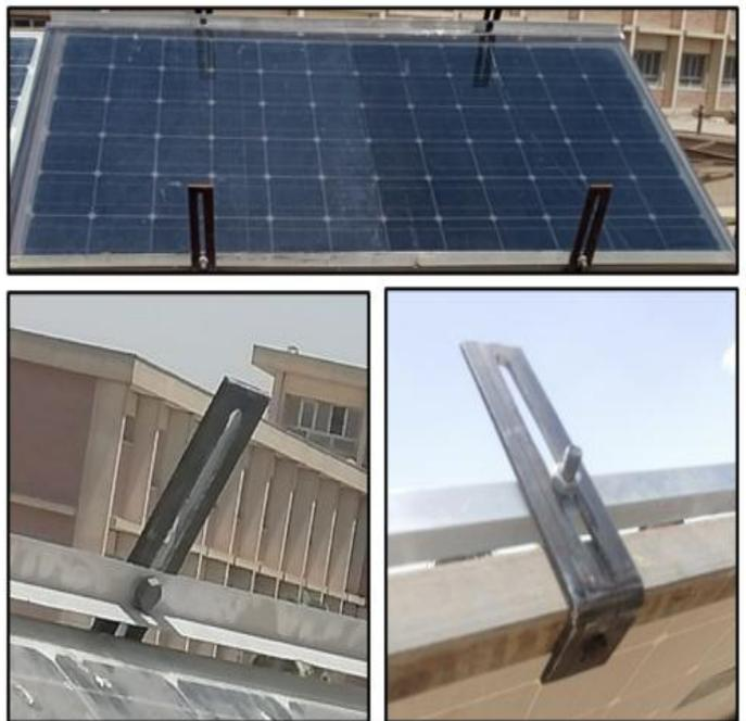
**Fig. 11** Fame-glass technique for cooling PV Panels (Panel D).
