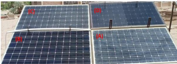
**Fig. 8** PV panels with different cooling techniques, (A) Reference panel; (B) Water-spray technique; (C) Iron-serpentine with water technique; and (D) Fame-glass technique.
