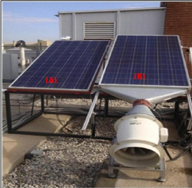
**Fig. 2** Air cooling techniques: (A) Natural, (B) Forced.
