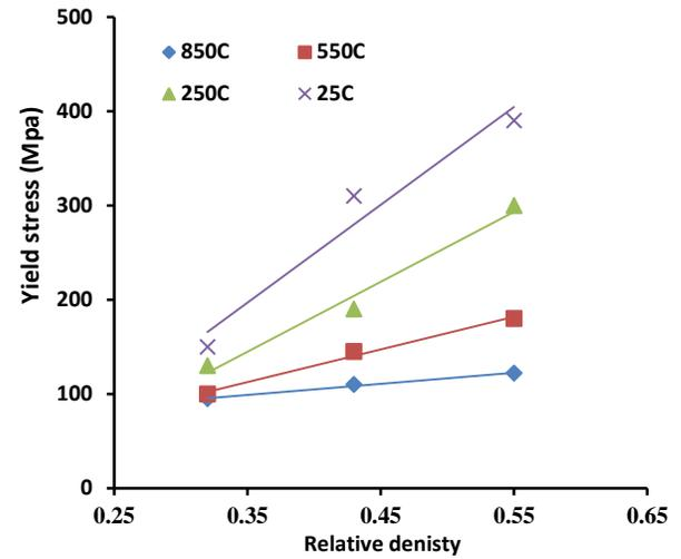
**Fig 4** variation in yield stress with respect to relative density and temperature of testing.
