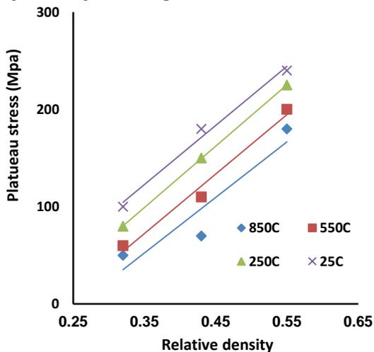
Fig. 6 Typical plateau stress versus density at various temperatures.
