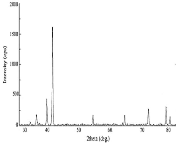
**Fig 3** XRD of titanium foam.
