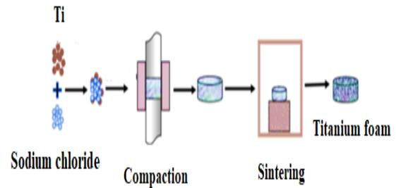
**Fig. 1** Processing of titanium foam.
