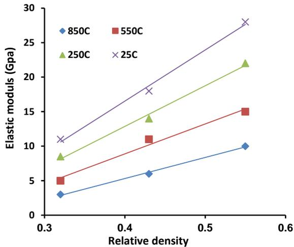
Fig 5 Modulus of elasticity vs relative density at a range of test temperatures.
