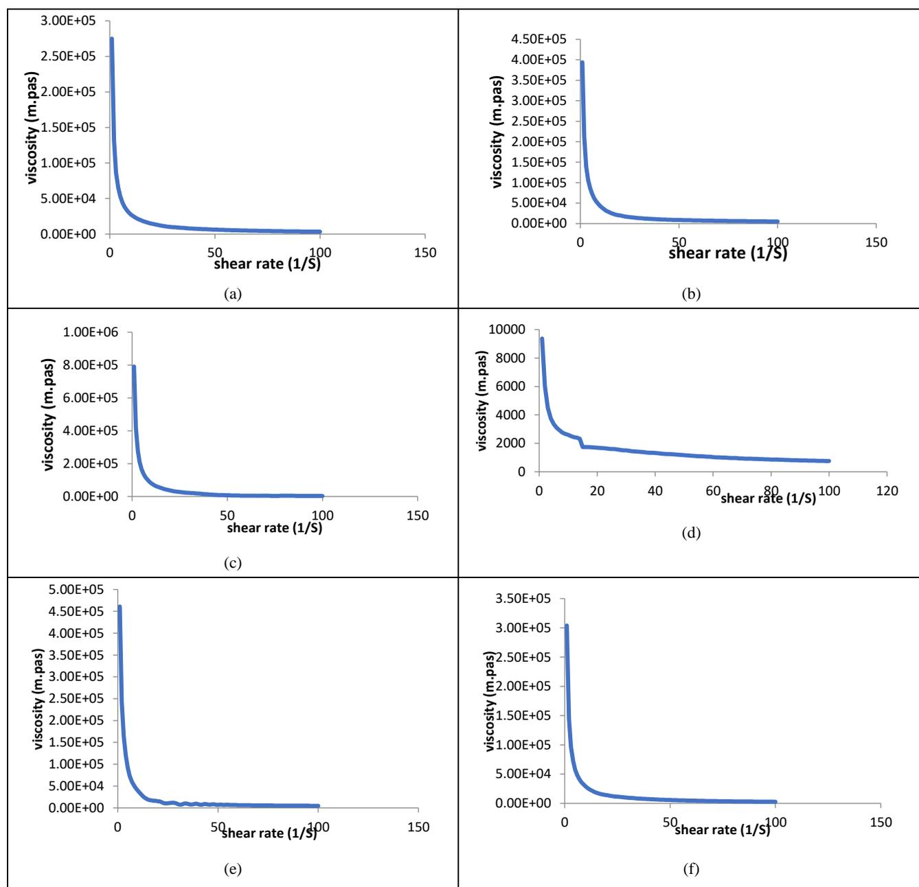
**Figure 7.** Relation between the dynamic viscosity and shear rate of (a) NG1, (b) NG2, (c) NG3, (d) NG4, (e) NG5 and (f) NG6
