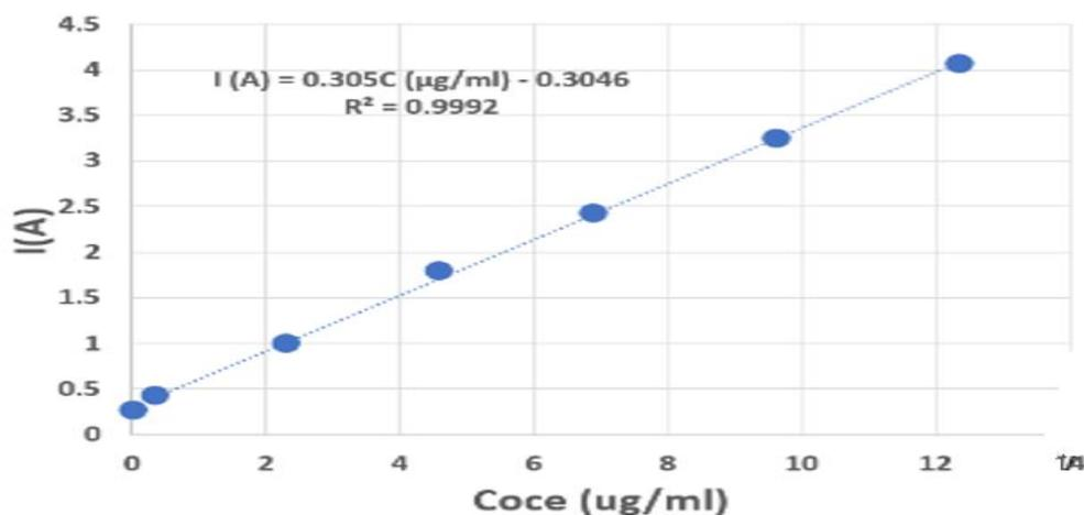
**Figure 6.** Calibration curve of peak Current of REBA to its Concentration at ZnO-NPs/CNTs/CPE.
