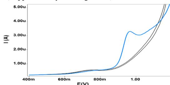
**Figure 3.** DP voltammograms (anodic peak responses) of REBA and its corresponding oxidative degradant at ZnONP/CNT/ME at pulse amplitude, 0.050 V; pulse time, 0.04 s; sweep rate, 0.050 V.s<sup>-1</sup>; voltage step, 0.005 V; and voltage step time, 0.1 s.
