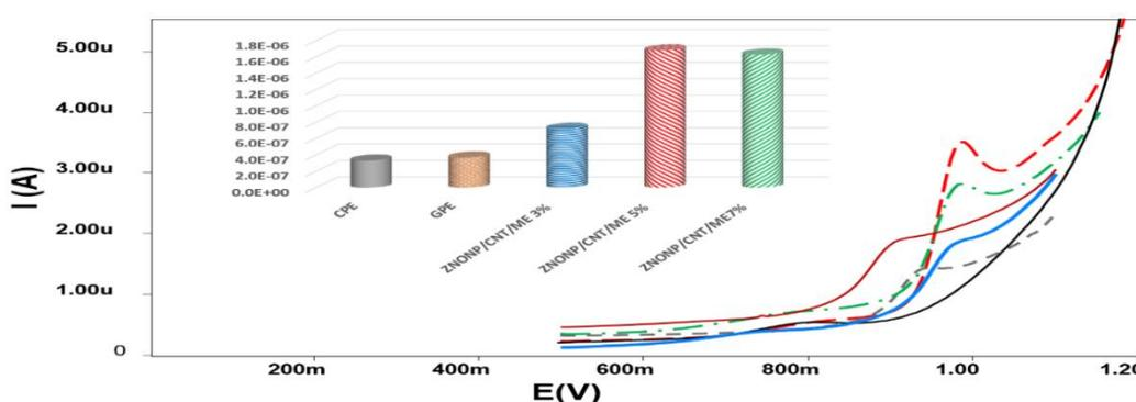
**Figure 2.** Comparative Behavior of Cyclic Voltammetric of REBA at working electrodes.
