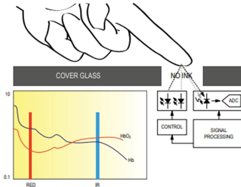
Fig. 2: SpO2 Sensor Working Principle. [19]
