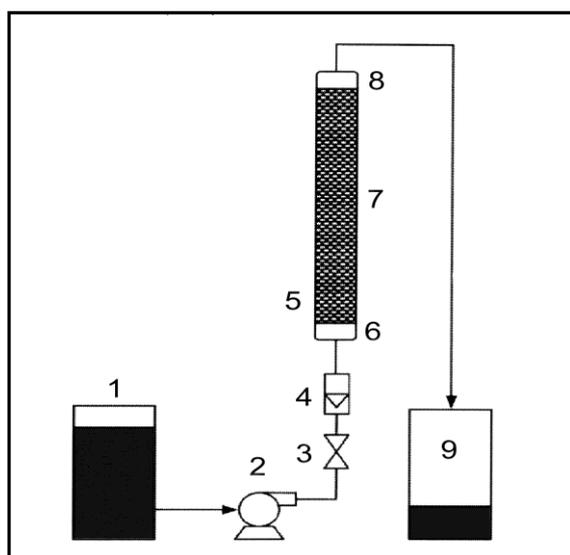
**Figure (1): Experimental arrangement of the removal packed bed column.**
