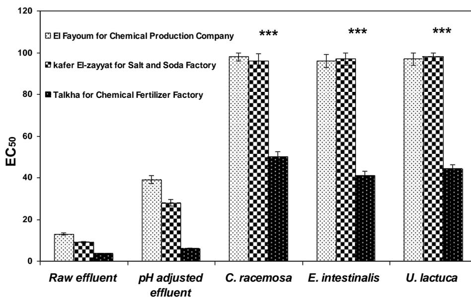
Figure (7): Efficiency of algal column to reduce toxicity of different industrial effluents.
