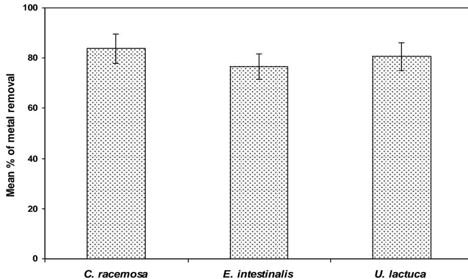
**Figure (5): Mean efficiency of algal column to remove different heavy metals. Error bars represent the standard errors of three replicates.**
