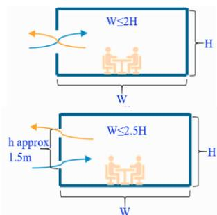
Fig. 9. Depth of the space compared to its height: single opening (top) – two openings (bottom) [33]
