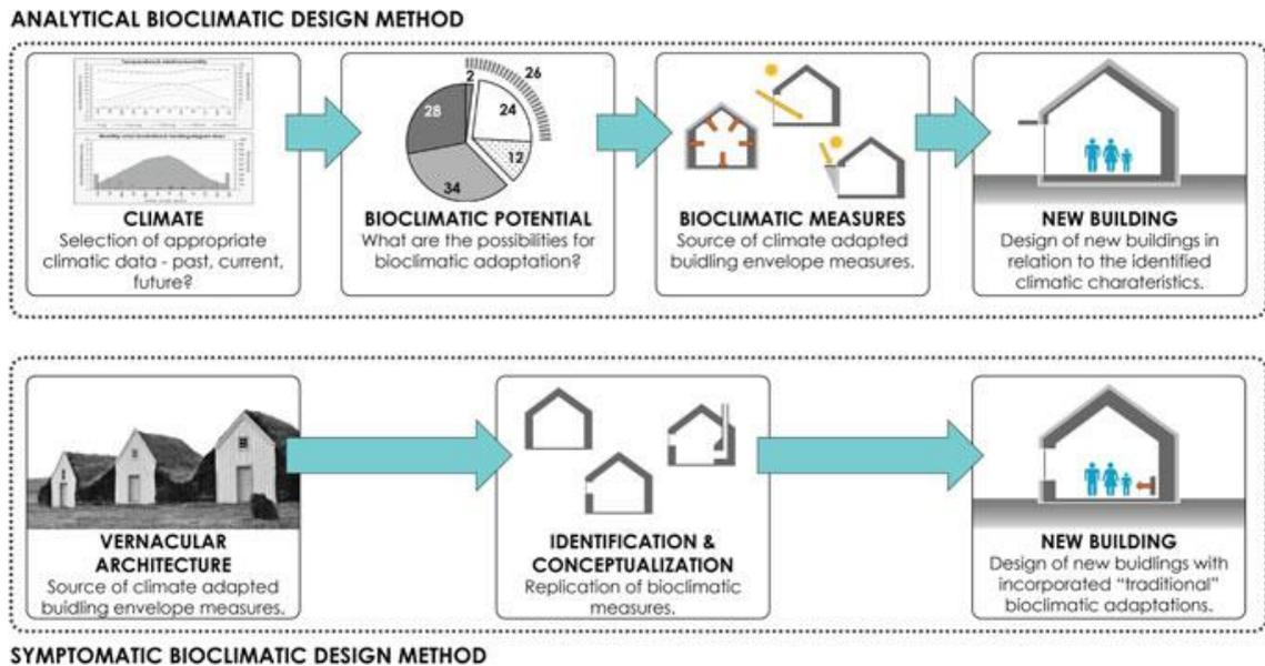
Fig. 3. Schematic representation of the design process for symptomatic (bottom) and analytical (top) methods of bioclimatic design [1]
