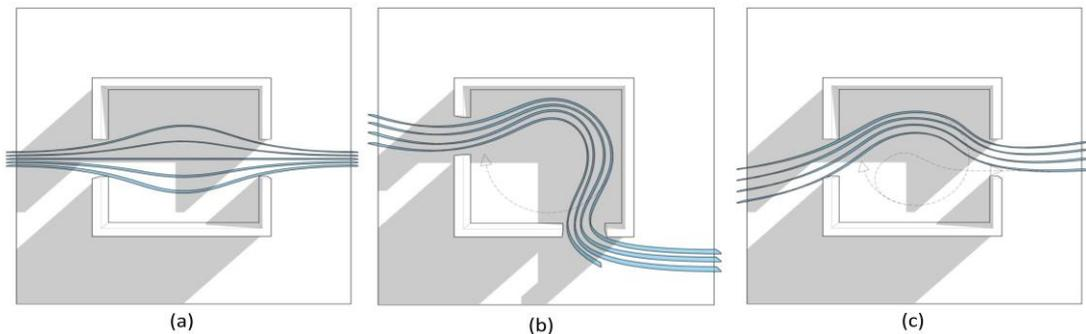
Fig. 20. Two opposite openings and vertical wind (a) - Two adjacent openings and vertical wind (b) - Two opposite openings and tilted wind (c) [Author]
