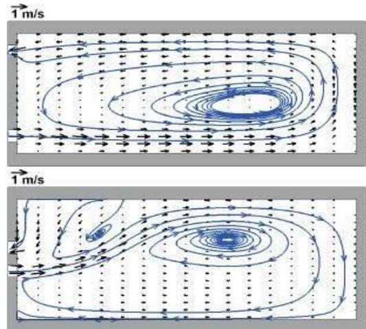
Fig. 10. Effect of the space between openings on air distribution inside spaces: wide-spaced (top) – close-spaced (bottom) [36]
