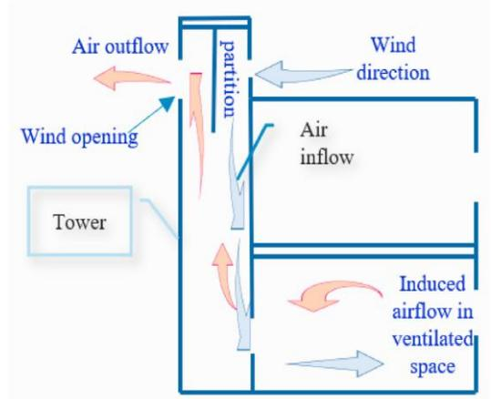
Fig. 14. Air movement inside wind catchers [33]
