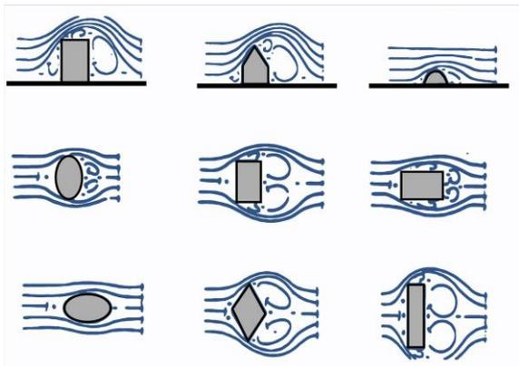
Fig. 19. Effect of building shape on wind pattern [54]
