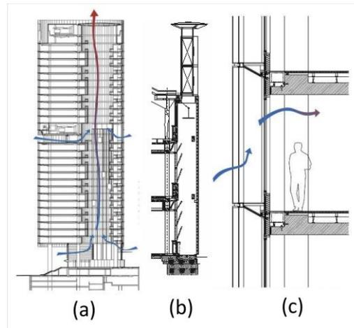
Fig. 15. Air movement through: atrium (a) – solar chimney (b) – double skin façade (c) [51, 52]
