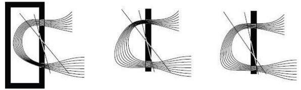
Fig. 8. Neutral level movement according to the opening area [36]
