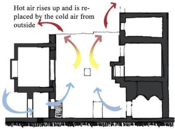
Fig. 16. Air movement inside the courtyard [35]
