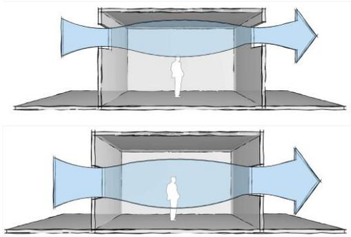
Fig. 21. High-level openings result in bad ventilation (top) - Two opposite openings at a human level for good ventilation (bottom) [Author]
