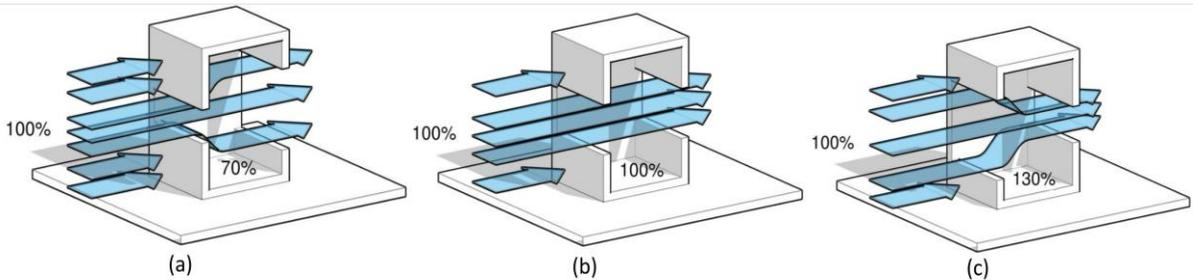
Fig. 22. Variation in air flow rates within a space due to variation in the air inlet and outlet size – (a) the inlet is smaller than the outlet – (b) the inlet and outlet are the same – (c) the inlet is bigger than the outlet size [Author]
