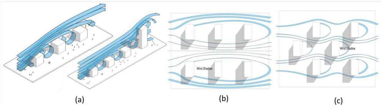
Fig. 18. The effect of buildings height on wind shadow pattern (a) – wind shadow of parallel urban pattern (b) – wind shadow of reciprocal urban pattern (c) [Author]
