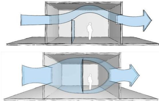
Fig. 23. The effect of partitions on wind direction – partition near inlet (top) – partition near outlet (bottom) [Author]
