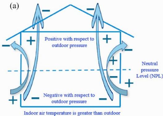
Fig. 7. Airflow caused by the stack effect [33]
