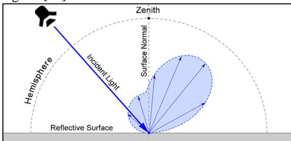
Figure 18: hemispheric reflection on the same side of the surface as the incident light. [11]
