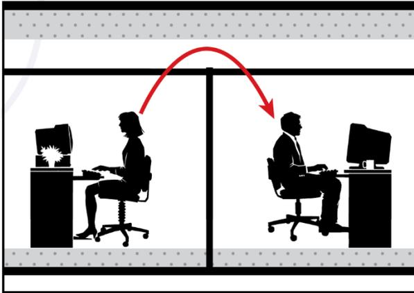
Figure 16: Sound transmission through a common plenum.
