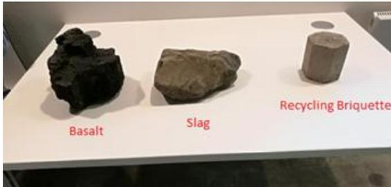
Figure 3: The essential components of rock wool tiles (Source: Technical training for the researcher 2018)
