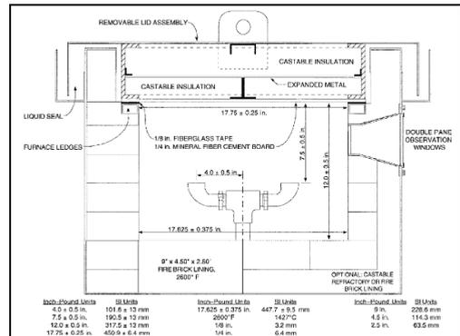
Figure 19: The Critical Dimensions of a Test Furnace (Not a Construction Drawing)
