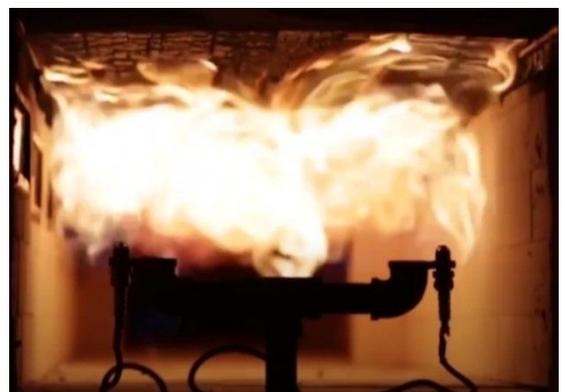
Figure 20: with the surface to be examined facing down toward the ignition source, the specimen is in the ceiling position [17].
