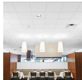
Figure 2: Photo of a mineral fiber suspended ceiling (Source: Armstrong Catalogue page 226)
