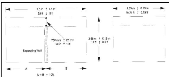
Figure 17: General Dimensions of the Test Room.
