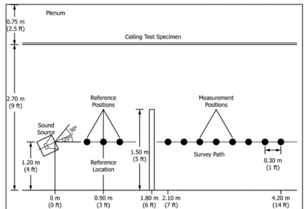
Figure 15: ceiling test facility according to ASTM E 1111
