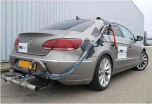
**Fig. 4.** Portable emissions measurement system [72].
