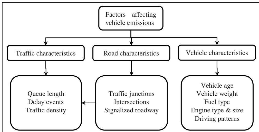
**Fig. 2.** The factors and characteristics vehicle emissions
