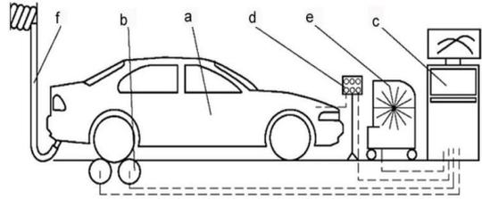
**Fig. 3.** Chassis dynamometer test stand [64].
