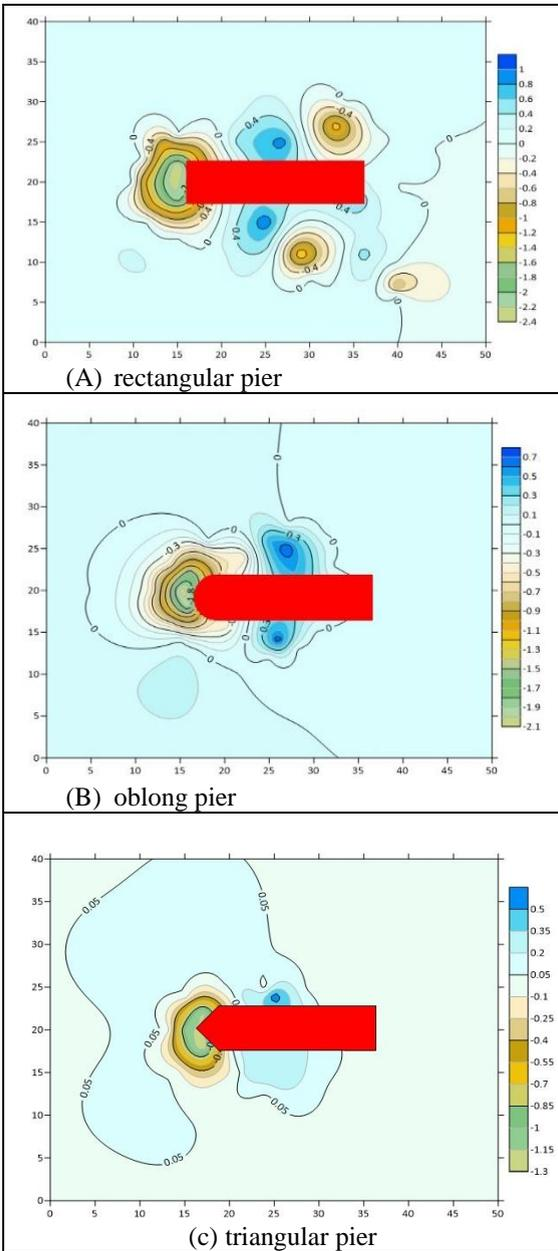
Figure 8: The contour map of bed morphology around all pier models without gabion nose for the flow velocity  $V = 0.267$  m/s.
