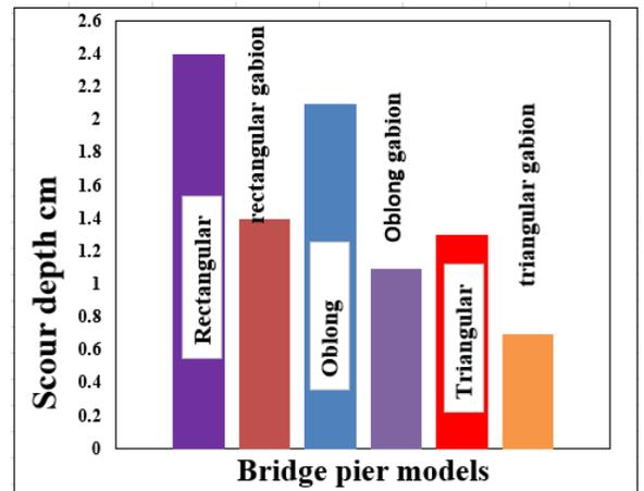
Figure 7: Scour around different bridge pier shapes and gabion noses for the flow velocity  $V = 0.267$  m/s.
