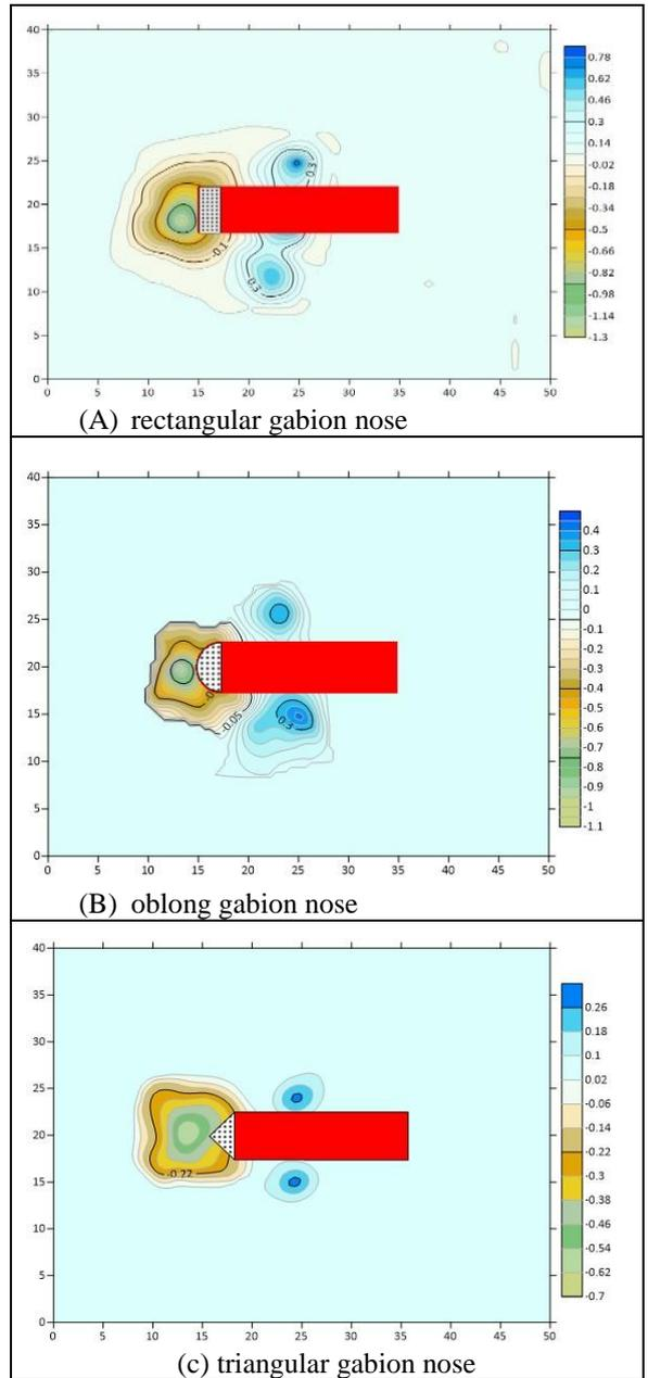
Figure 9: The contour map of bed morphology around pier model's with gabion nose for the flow velocity  $V = 0.267$  m/s.
