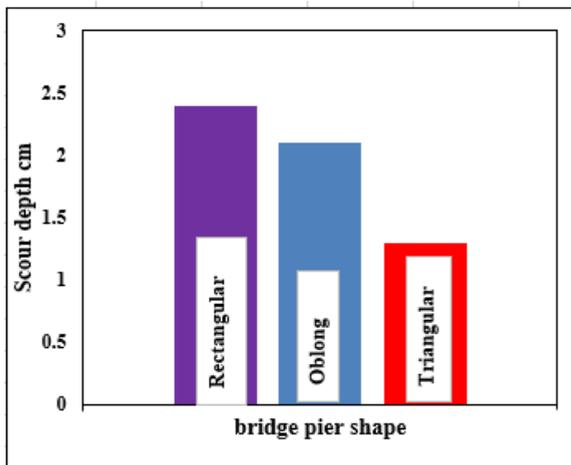
Figure 5: Scour around different bridge pier shapes for the flow velocity  $V = 0.267$  m/s.
