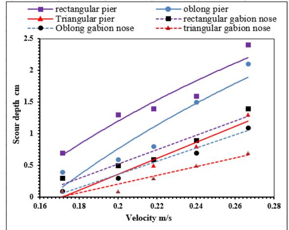
Figure 6: The relationship between velocity and scour depth of different pier models
