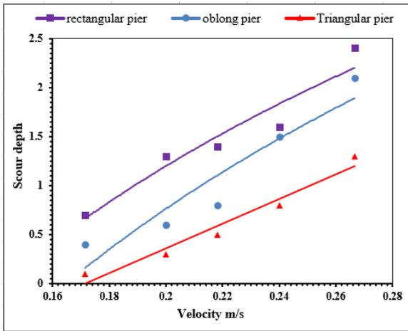
Figure 4: The relationship between velocity and scour depth of different uniform pier shapes
