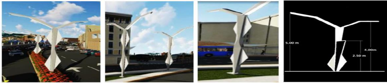
Fig.16- (1-2): The lighting units were designed in a simple way to suit the design of the place where it works with a hybrid energy system, using electricity in addition to panels and solar cells for the optimal use of sunlight in the area .
