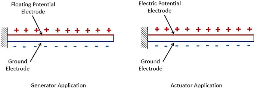
Fig. 4 Piezoelectric material electrodes identification on COMSOL Multiphysics.
