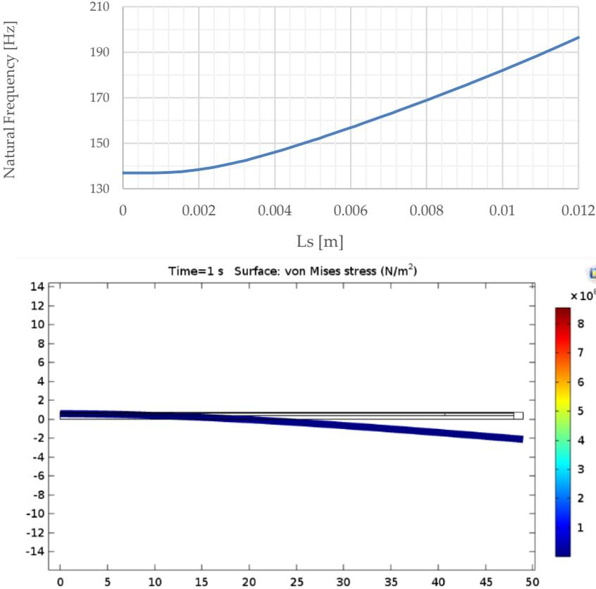
Fig. 7 (a) Relation from COMSOL Multiphysics model between support position from root ( $l_s$ ) and natural frequency of beam, (b) Numerical model simulation, live video, [11].
