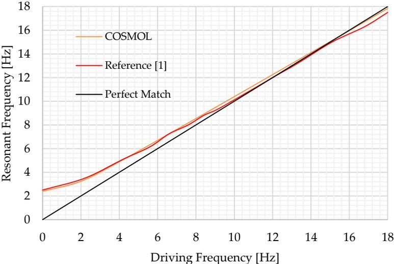
**Fig. 4 Data comparison between finite element numerical model and perfect match line.**
