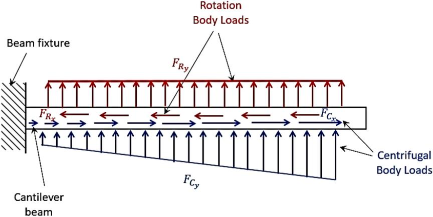
Fig. 1 Effect identification of the different force across the harvester on COMSOL Multiphysics.
