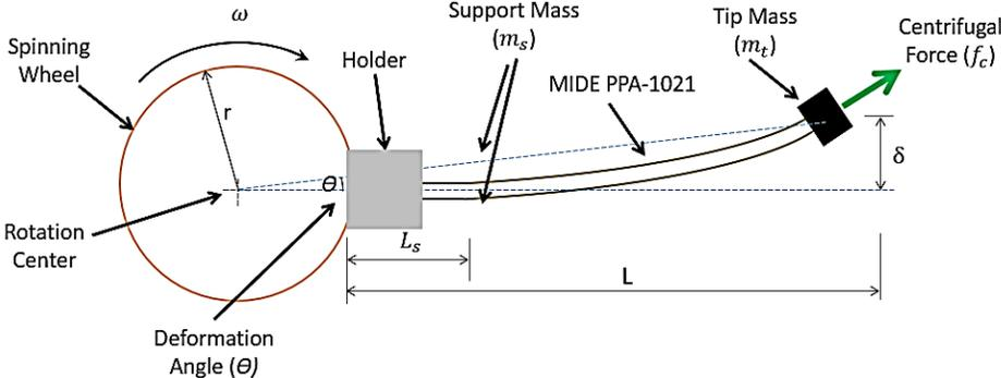
**Fig. 1 Harvester detailed construction.**
