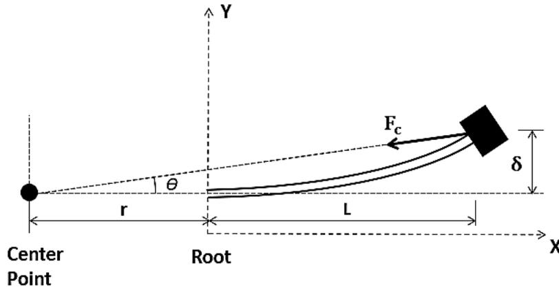
Fig. 3 Effect of centrifugal force on beam tip deflection.
