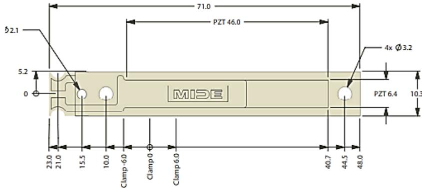
**Fig. 2 Detailed dimensions for MIDE PPA-1021 and layers composition.**
