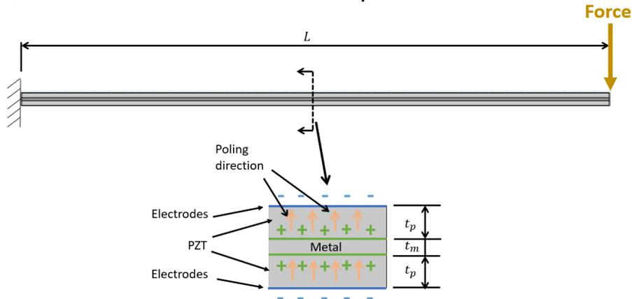
Fig. 10 A schematic for the modeled triple-layer bender on COMSOL Multiphysics.
