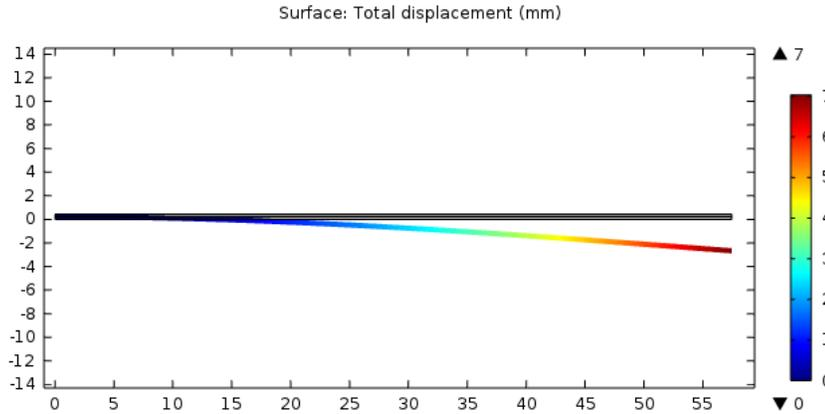
**Fig. 6 Simulated tip deformation mm due to applied tip force N and voltage difference (V) on numerical model.**
