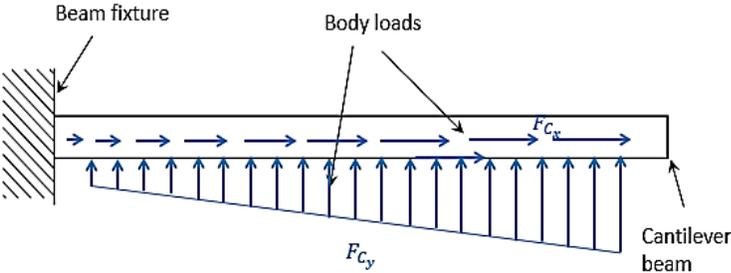
Fig. 2 Centrifugal forces identification across the harvester on COMSOL Multiphysics.
