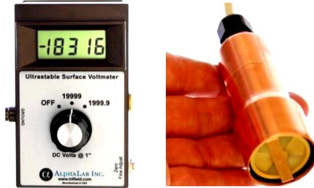
Fig. 1 Electrostatic field measuring device.
