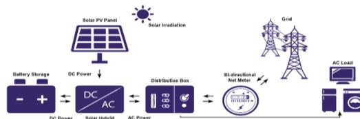
Fig. 9 Hybrid PV system, [8].
