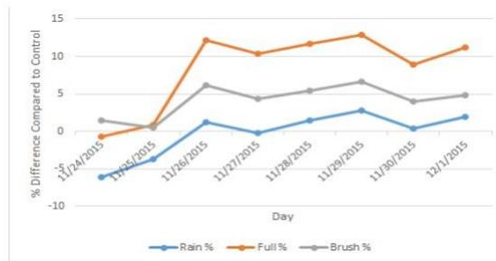
Fig. 11 Improvement in solar energy generation after cleaning, [3].
