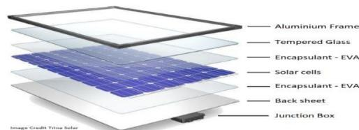
Fig. 2 Structure of the Solar Panel
