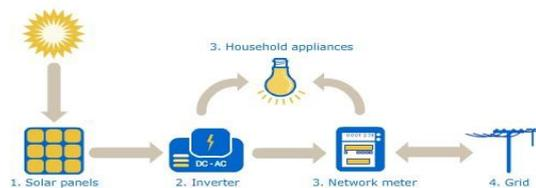
Fig. 14 Major PV Solar System Component.
