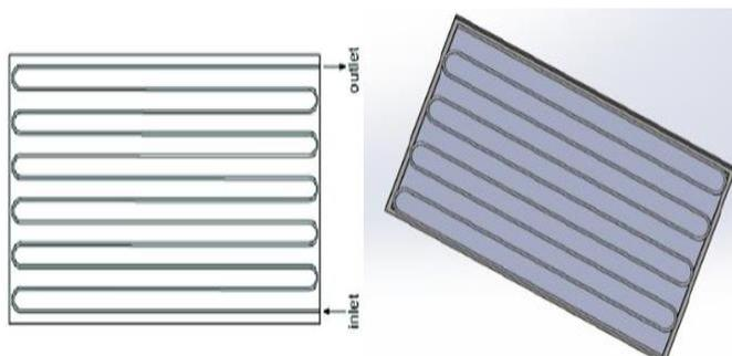
**Fig. 28 Cooling serpentine tube.**
