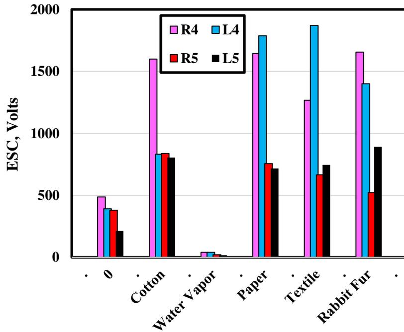
Fig. 6 ESC generated on the surface of the lenses of goggles after rubbing by different materials.
