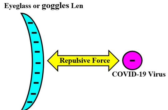
Fig. 11 Illustration of the repulsive force between the eyeglass lens and negatively charged viruses.
