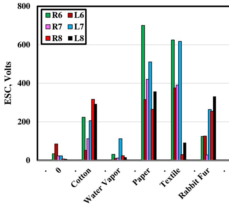
Fig. 7 ESC generated on the surface of the lenses of goggles after rubbing by different materials.
