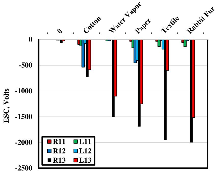
Fig. 9 ESC generated on the surface of the lenses of goggles after rubbing by different materials.
