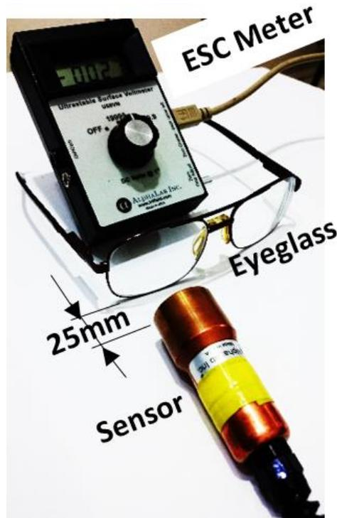
**Fig. 2 Measuring Procedure.**
