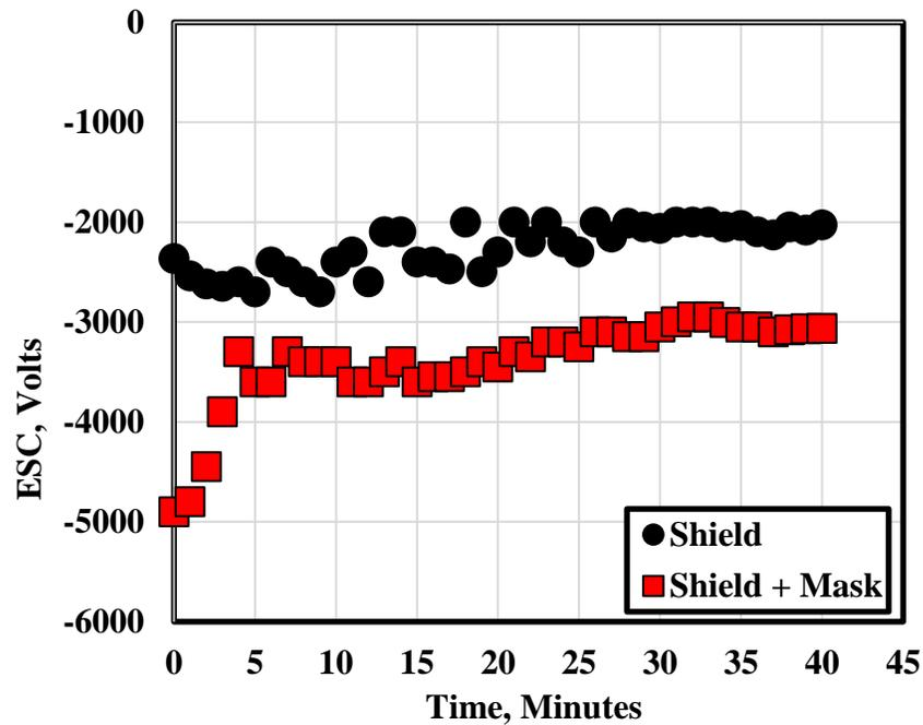
Fig. 3 ESC generated on the surface of face shield versus time.
