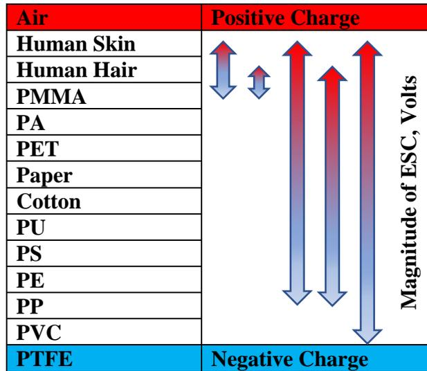
Fig. 4 Triboelectric series of the proposed materials.
