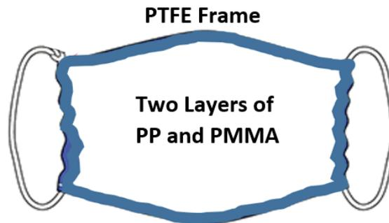
Fig. 6 Framing the mask by PTFE.
