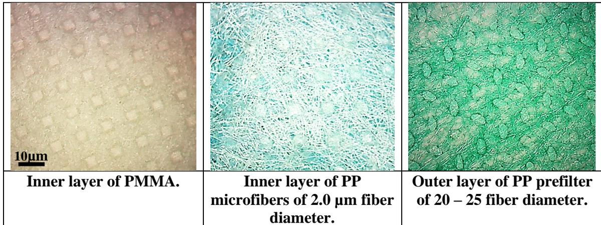
Fig. 2 Optical microscopes of the proposed material for the face mask.
