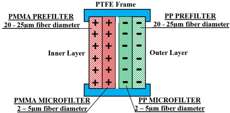
Fig. 1 Cross section of the proposed surgical mask.
