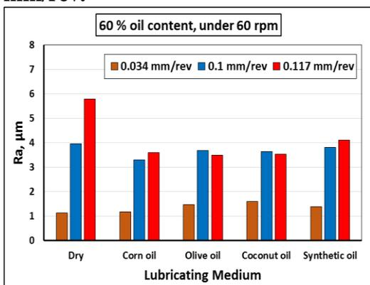
**Fig. 3** effect of oil type and feed rate on surface roughness of Al. under 60 rpm and 60 % oil content
