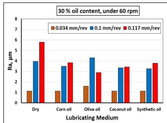
**Fig.2** effect of oil type and feed rate on surface roughness of Al. under 60 rpm and 30 % oil content
