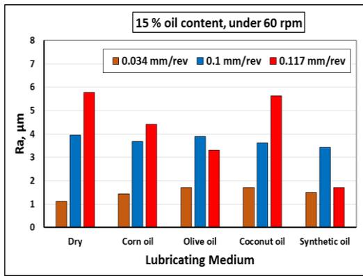
**Fig.1** effect of oil type and feed rate on surface roughness of Al. under 60 rpm and 15 % oil content
