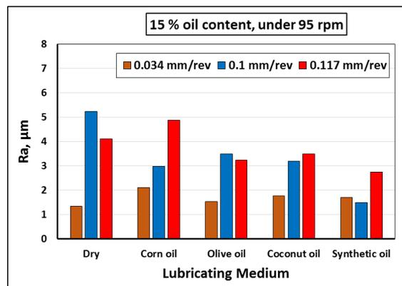
**Fig. 4** effect of oil type and feed rate on surface roughness of Al. under 95 rpm and 15 % oil content
