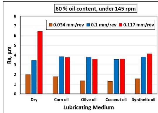
**Fig. 9** effect of oil type and feed rate on surface roughness of Al. under 145 rpm and 60 % oil content
