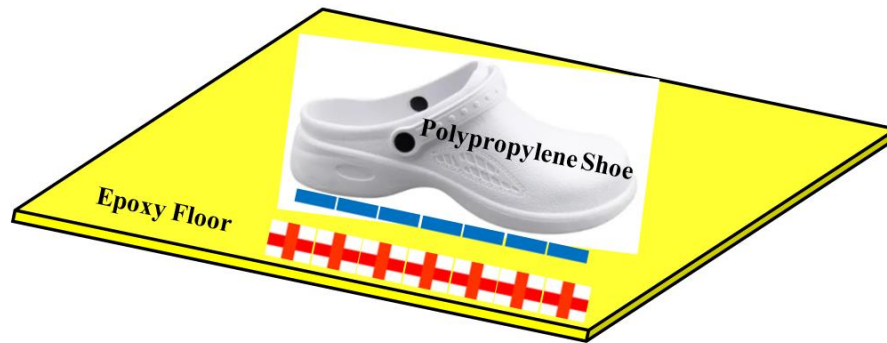
Fig. 12 Generation of ESC on the sliding surfaces of PP shoe and epoxy floor.
