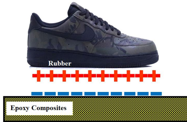
Fig. 11 Generation of ESC on the sliding surfaces of rubber shoe and epoxy floor.
