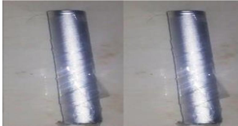
**Fig. 1 Aluminum foil mold in cylindrical shape.**
