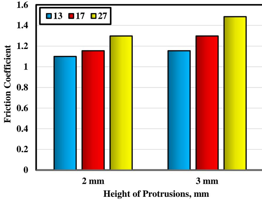
Fig. 7 Friction coefficient displayed by rubber protrusions of 3 mm diameter.
