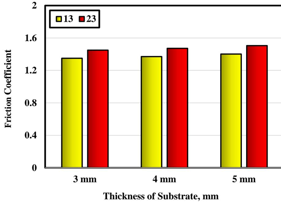
Fig. 11 Friction coefficient displayed by rubber protrusions of 5 mm diameter.
