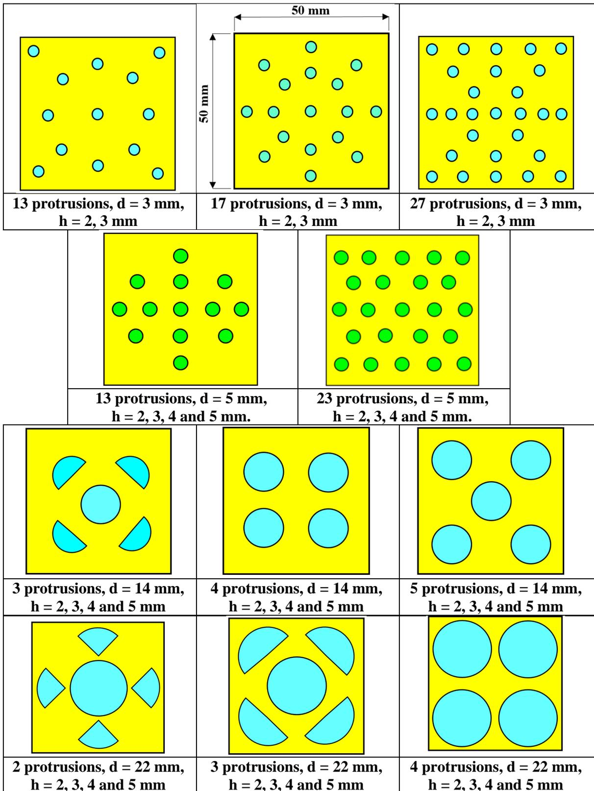
Fig. 2 Details of the rubber protrusions.
