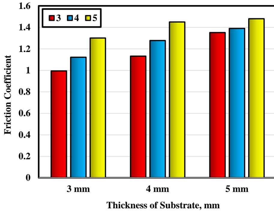
Fig. 10 Friction coefficient displayed by rubber protrusions of 14 mm diameter.
