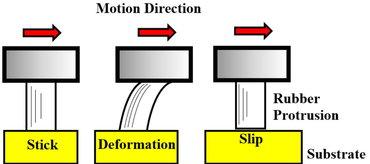
Fig. 8 Illustration of the mechanism of friction rubber.
