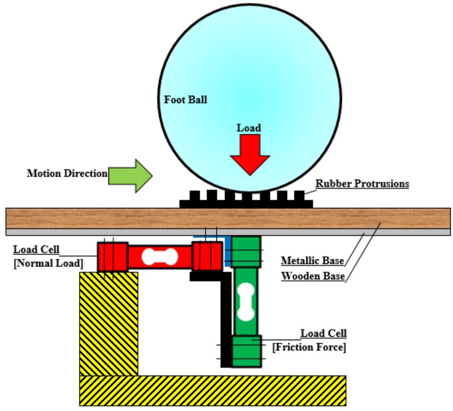
Fig. 1 Arrangement of the test rig.
