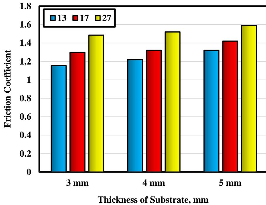
Fig. 12 Friction coefficient displayed by rubber protrusions of 3 mm diameter.
