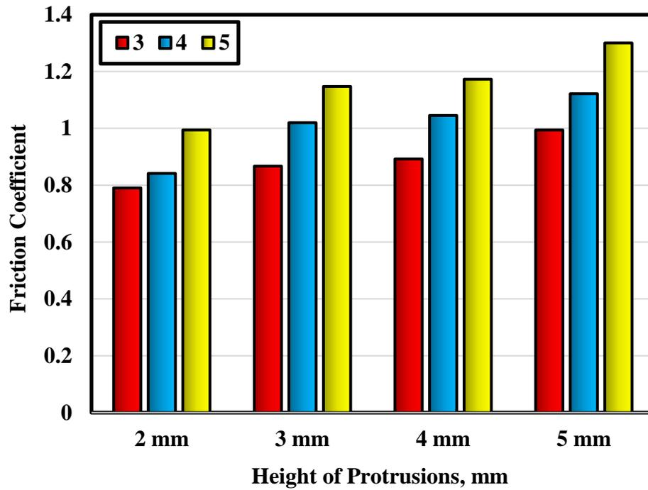
Fig. 5 Friction coefficient displayed by rubber protrusions of 14 mm diameter.
