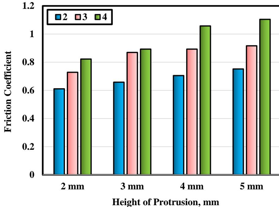
Fig. 4 Friction coefficient displayed by rubber protrusions of 22 mm diameter.
