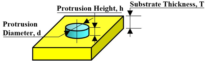
Fig. 3 Test specimens.
