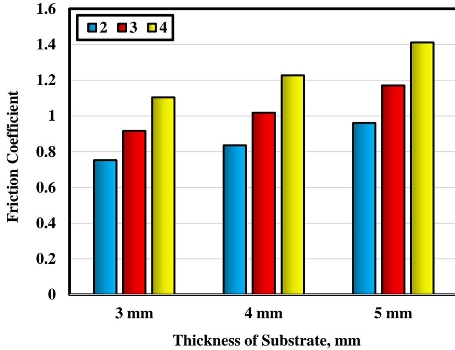
Fig. 9 Friction coefficient displayed by rubber protrusions of 22 mm diameter.
