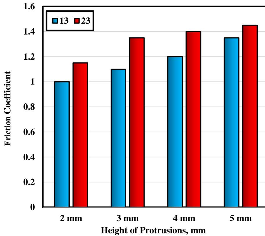
Fig. 6 Friction coefficient displayed by rubber protrusions of 5 mm diameter.
