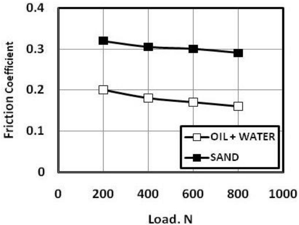
Fig. 17 Friction coefficient of oil and water lubricated sliding of rubber square protrusions against ceramic tiles.
