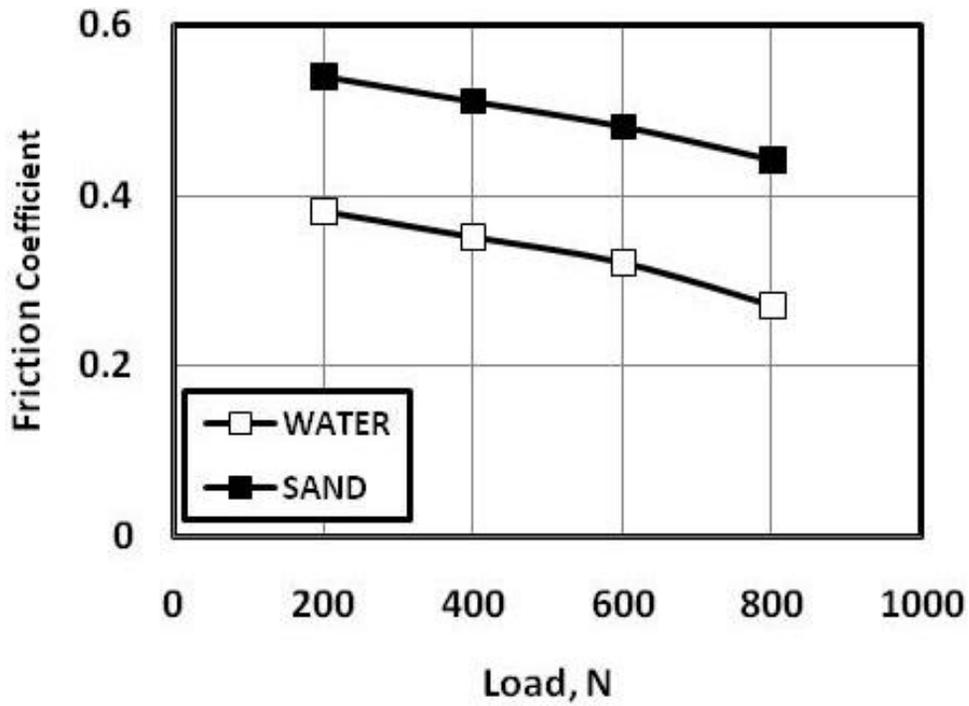
Fig. 8 Friction coefficient of water lubricated sliding of rubber square protrusions against ceramic tiles.
