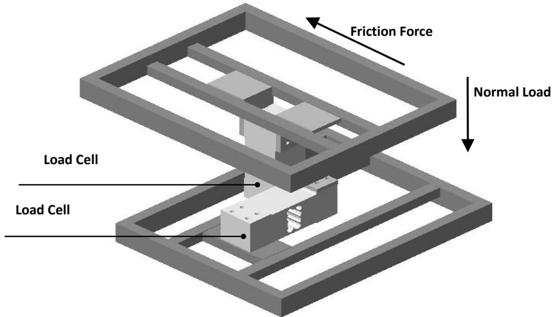
**Fig. 1 Basic features of the test rig.**
