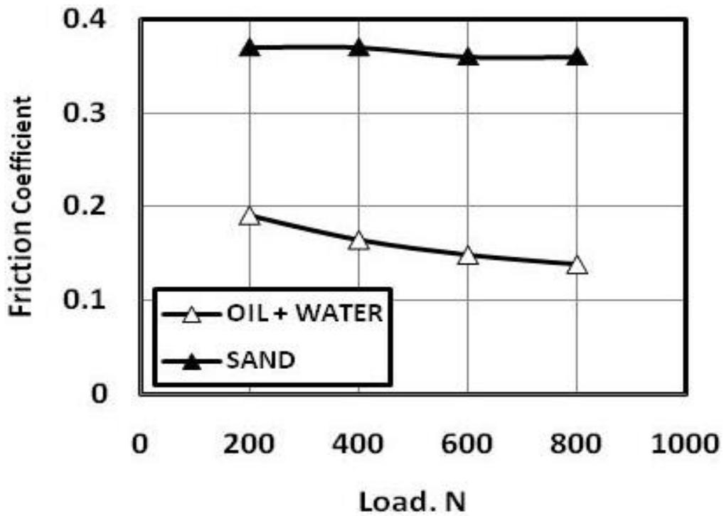
Fig. 15 Friction coefficient of oil and water lubricated sliding of flat rubber against ceramic tiles.
