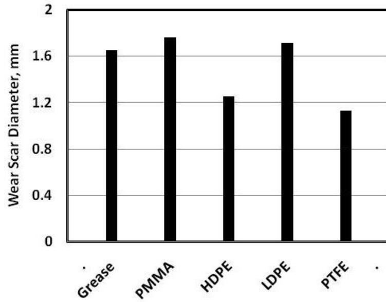
Fig. 6 Wear scar width caused by grease contaminated by iron ore.
