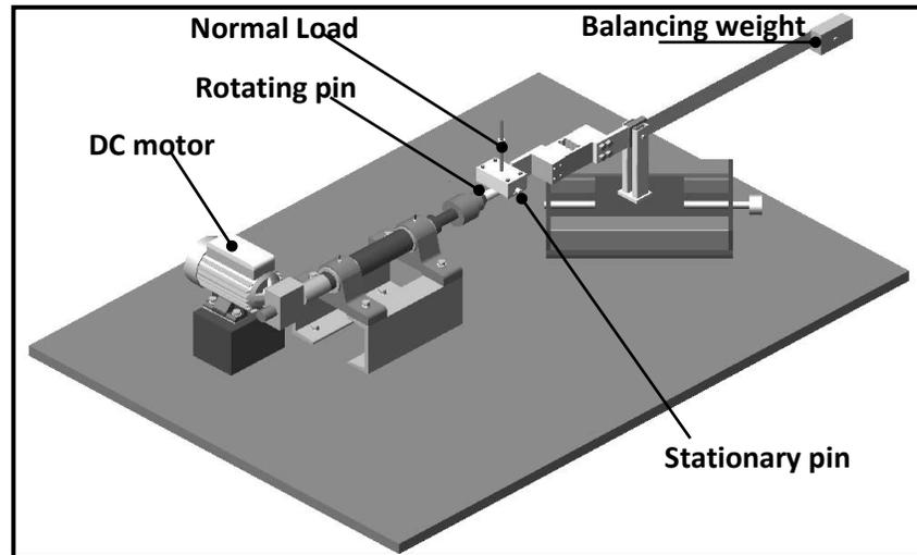
Fig. 1 Arrangement of the test rig.
