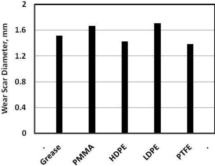
Fig. 3 Wear scar width caused by grease contaminated by sand clay.
