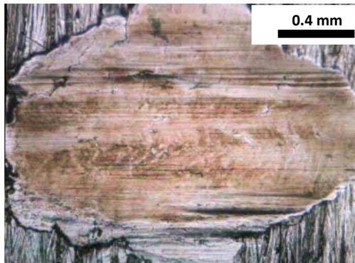
**Fig. 11** Photomicrograph of the wear scar diameter caused by grease contaminated by sand clay.
