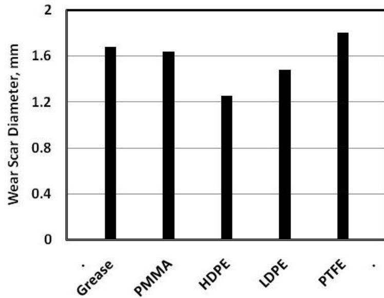
Fig. 7 Wear scar width caused by grease contaminated by limestone.
