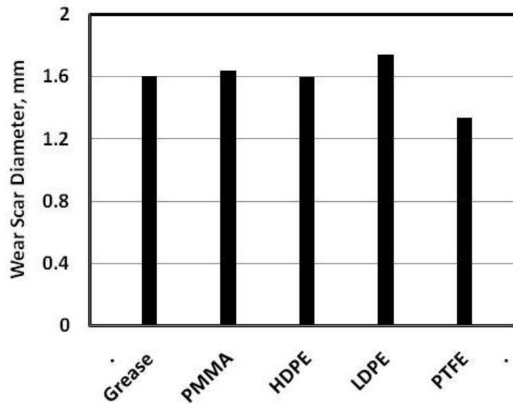
Fig. 5 Wear scar width caused by grease contaminated by air cooled slag (low ferric particles).
