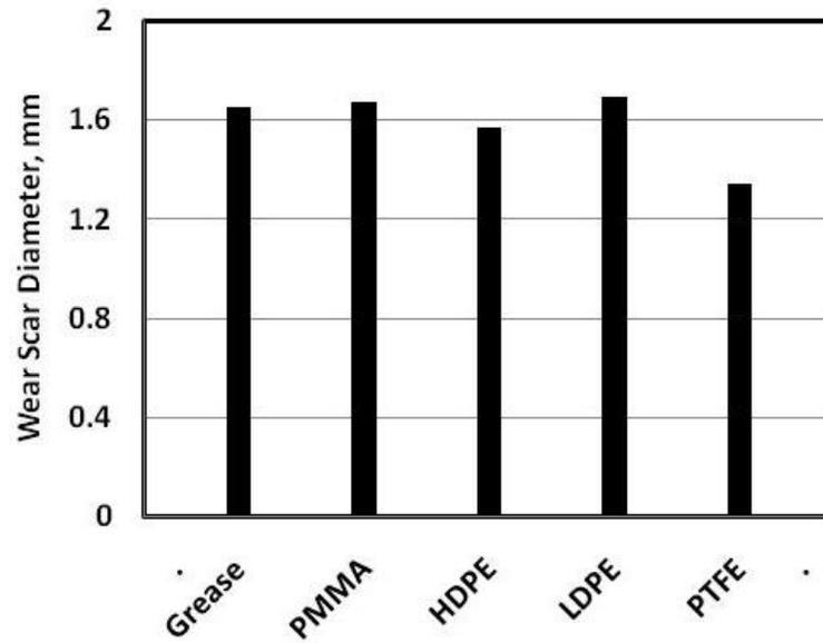
Fig. 8 Wear scar width of test specimens caused by grease contaminated by fatty clay.
