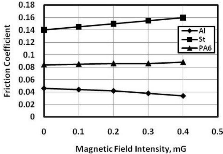
Fig. 7 Friction coefficient displayed by the sliding of steel pin against tested materials lubricated by oil dispersed by graphite.
