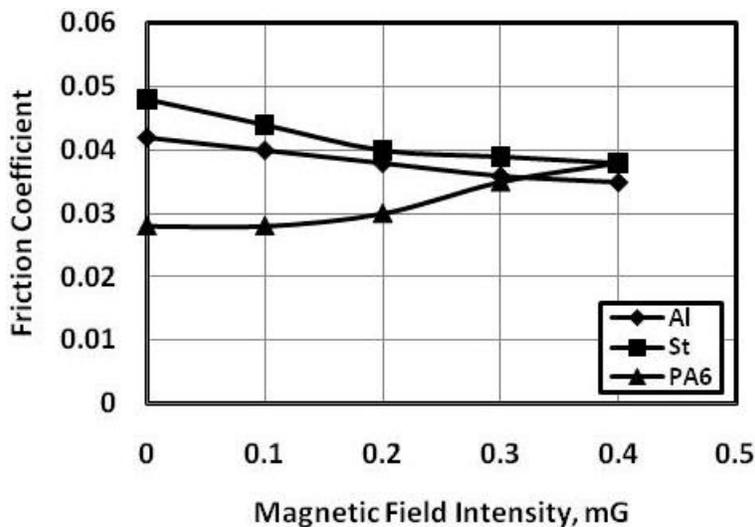
**Fig. 6 Friction coefficient displayed by the sliding of steel pin against tested materials lubricated by oil dispersed by CMOC.**
