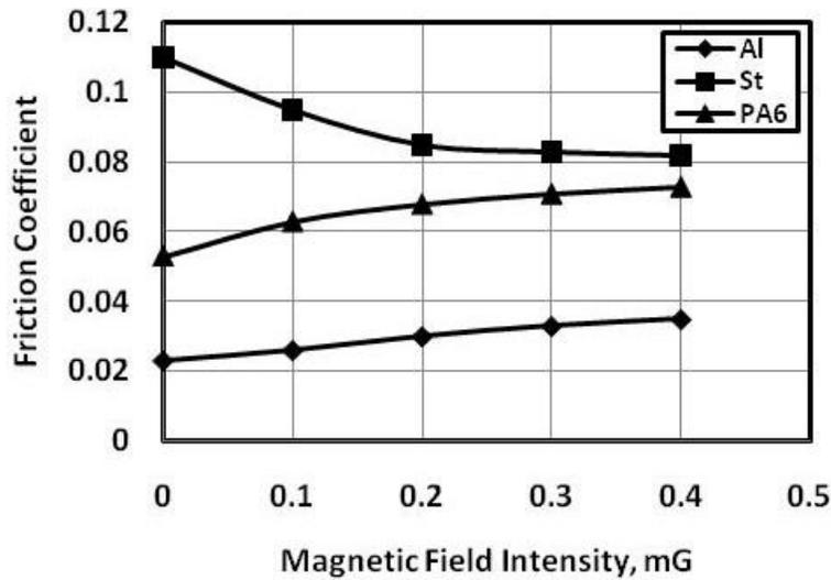
**Fig. 5 Friction coefficient displayed by the sliding of steel pin against tested materials lubricated by oil dispersed by MoS<sub>2</sub>.**
