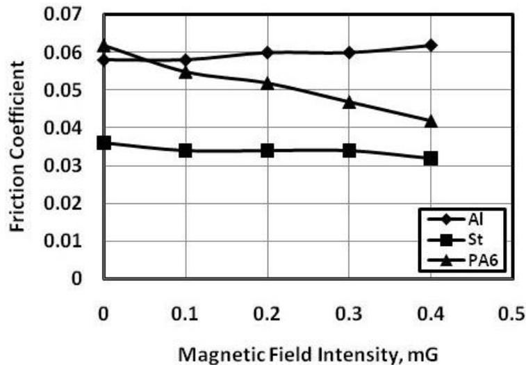
**Fig. 10 Friction coefficient displayed by the sliding of steel pin against tested materials lubricated by oil dispersed by PMMA.**
