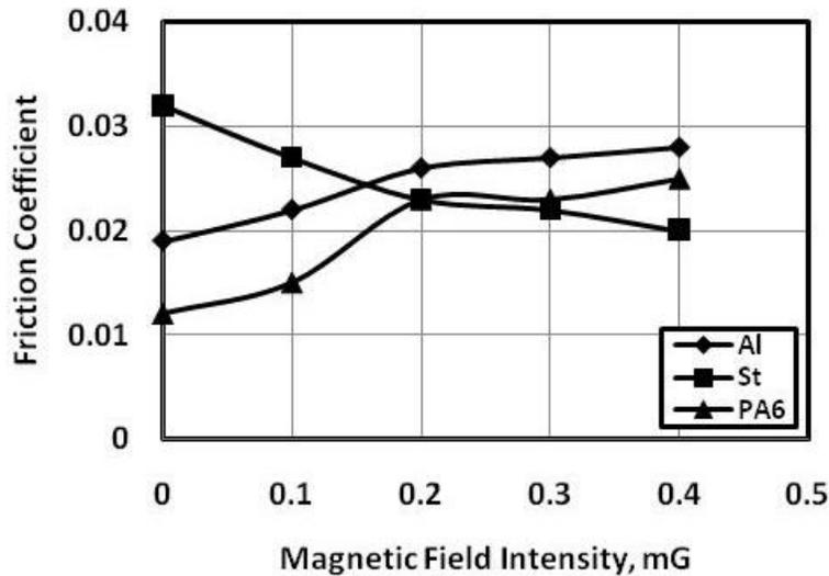
Fig. 9 Friction coefficient displayed by the sliding of steel pin against tested materials lubricated by oil dispersed by PTFE.
