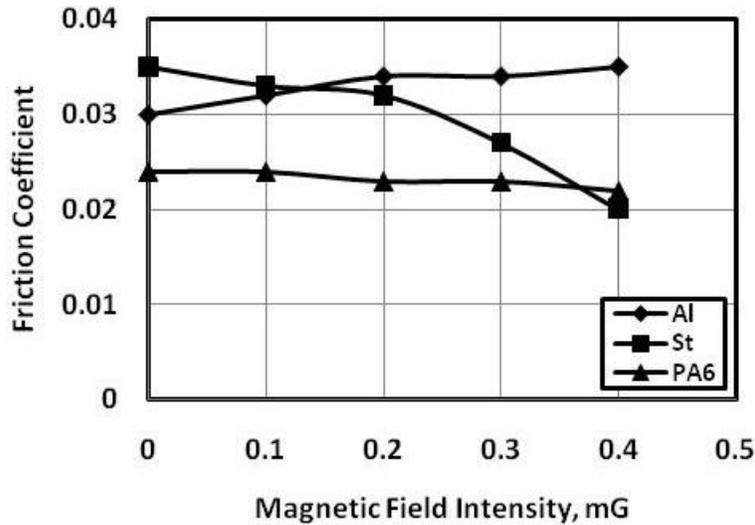
Fig. 8 Friction coefficient displayed by the sliding of steel pin against tested materials lubricated by oil dispersed by DA.
