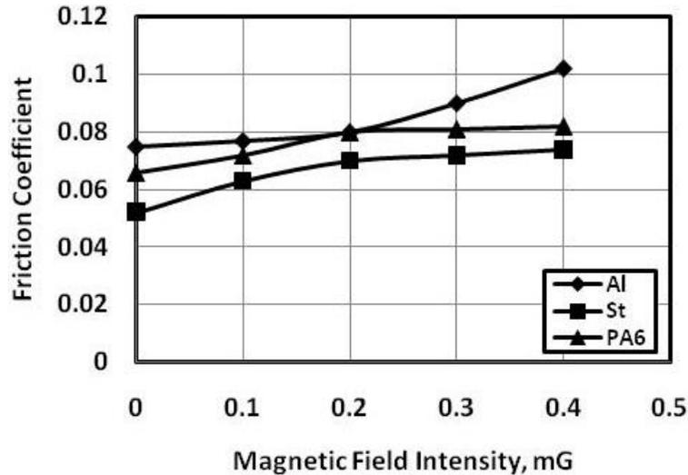
Fig. 3 Friction coefficient displayed by the sliding of steel pin against oil lubricated tested materials.
