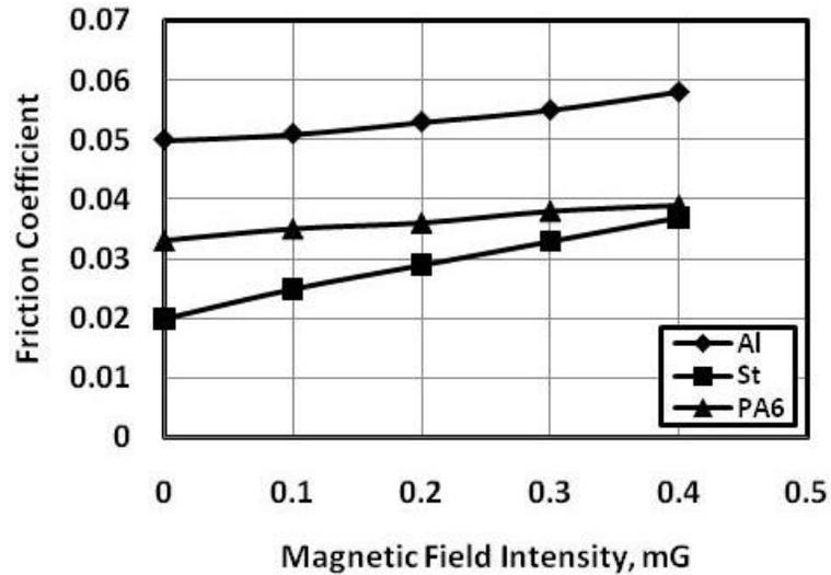
**Fig. 4 Friction coefficient displayed by the sliding of steel pin against tested materials lubricated by oil dispersed by ZDDP.**
