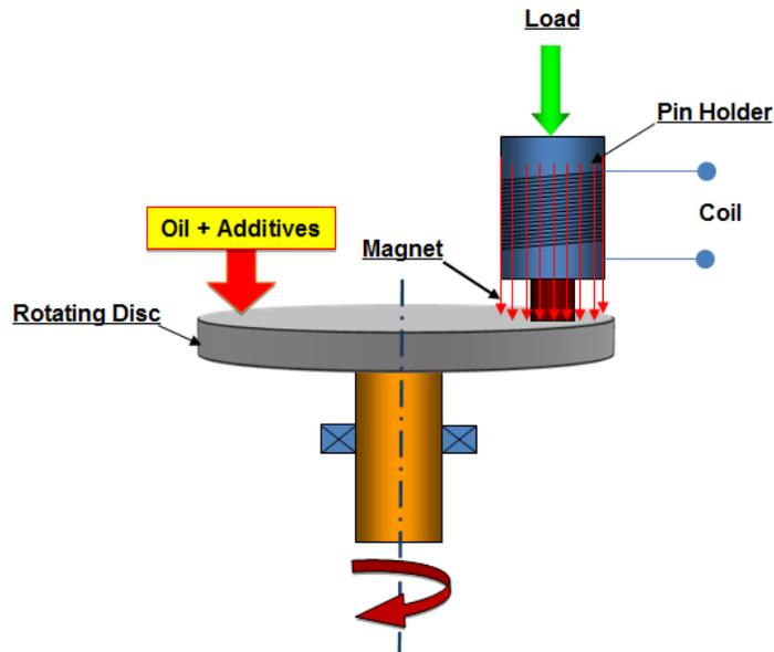
**Fig. 2 Application of the magnetic field.**
