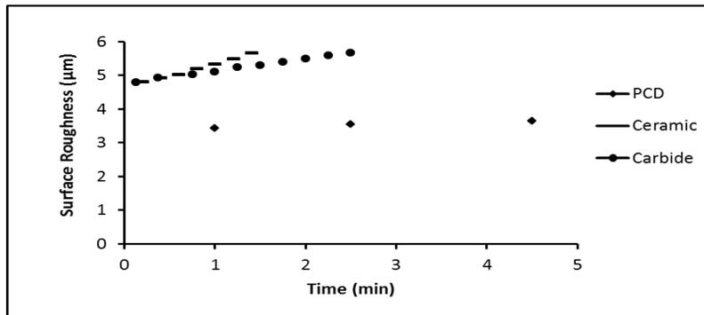
**Fig. 8 Surface roughness-Time curves for different tool materials**
