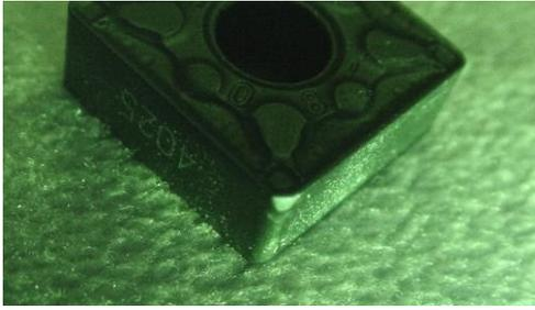
**Fig. 5 Carbide edge at 0.7 mm flank wear**
