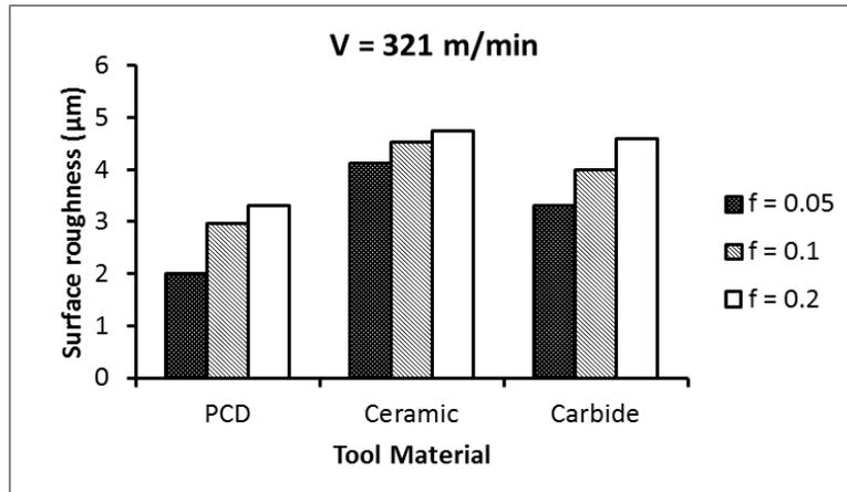
Fig. 13 Influence of tool material on surface roughness of composite at different feeds.
