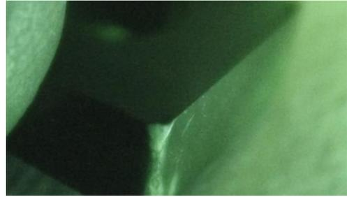
**Fig. 6 Ceramic edge at 0.7 mm flank wear**
