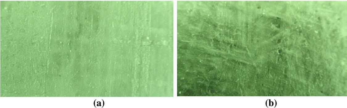
**Fig. 9 Composite material after cut using PCD Tool (scale 5:2).**
