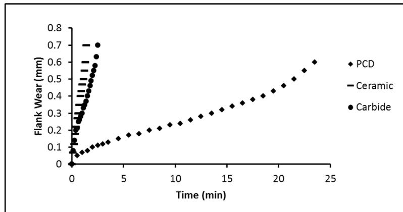
Fig. 4 Wear curves for different tool materials
