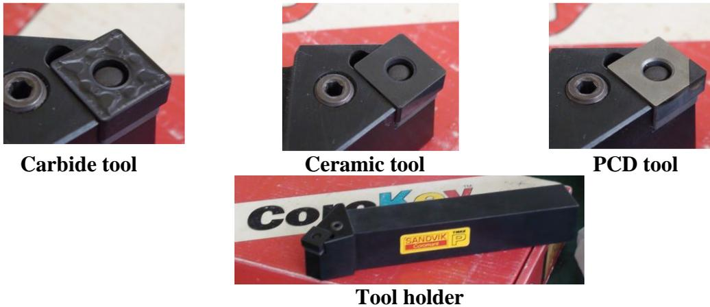
Fig. 1 The three different tool materials with the tool holder.
