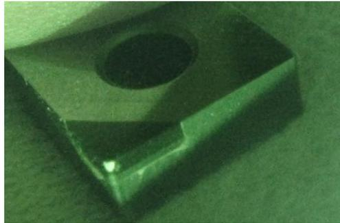
**Fig. 7 PCD edge at 0.6 mm flank wear.**
