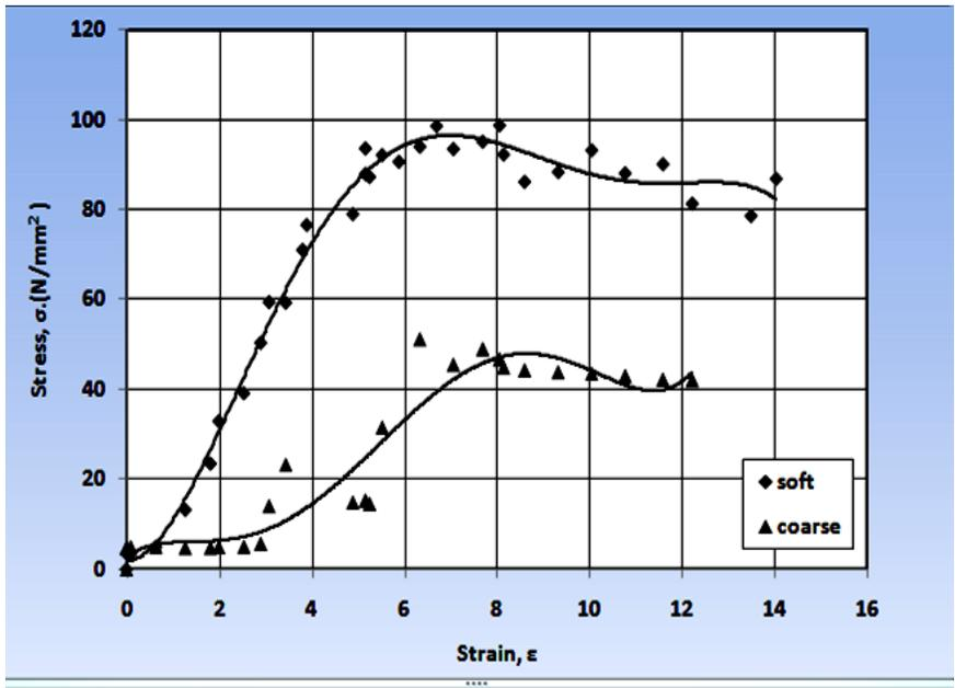
Fig. 8 Stress–strain curve for polyester composites filled by 30 wt. % jasmine. eaves.
