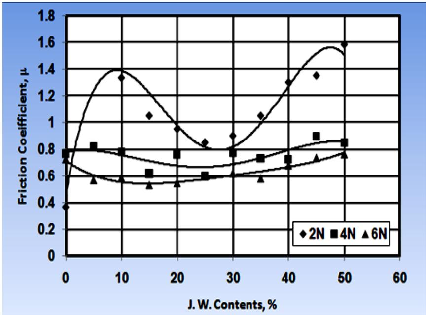
Fig. 4 Effects of coarse particles of jasmine leaves on the friction coefficient of polyester composite.
