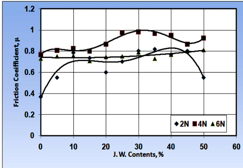
Fig. 3 Effects of soft particles of jasmine leaves on the friction coefficient of polyester composite.
