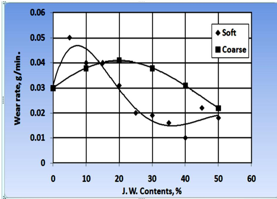
Fig. 5 Effects of jasmine leaves on wear rates of polyester composite.
