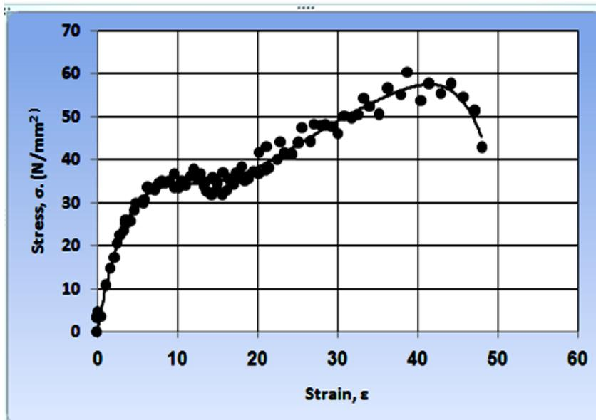
Fig. 6 Stress – strain curve for polyester free of jasmine leaves.
