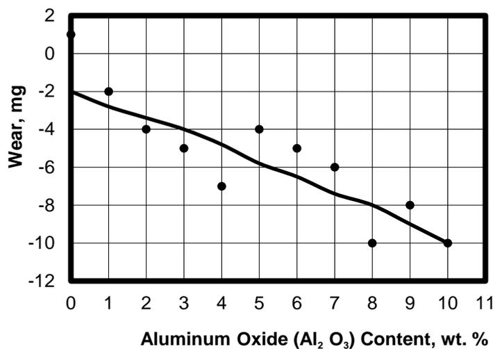
**Fig. 21** Effect of aluminum oxide nanopowder on wear of PE filled by 9 wt. % oil content.
