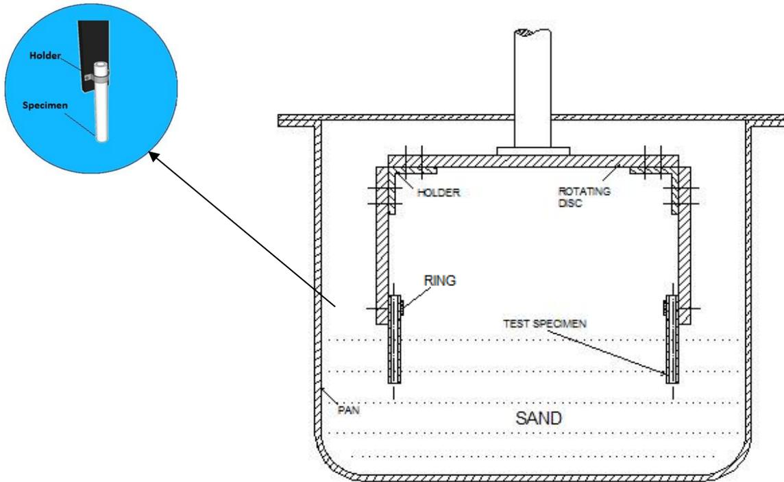
**Fig. 2 Layout of Sand Test Rig, [14].**
