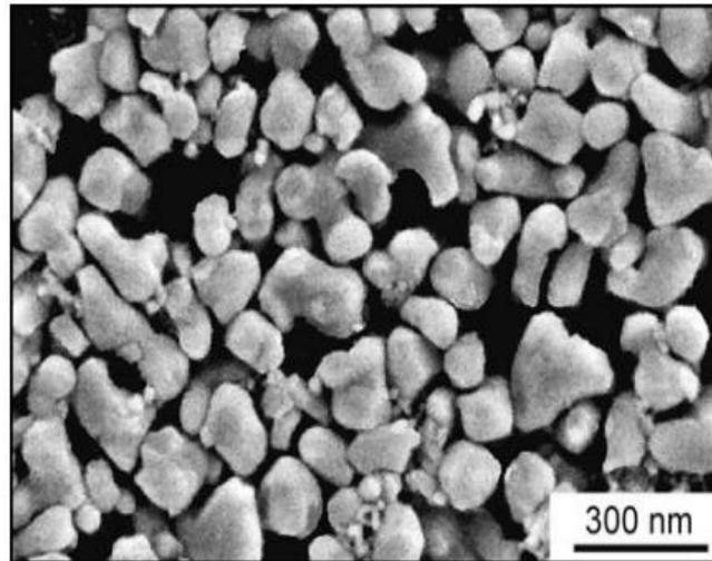
**Fig. 3 SEM micrograph of the  $\text{Al}_2\text{O}_3$  nanopowder, [15].**
