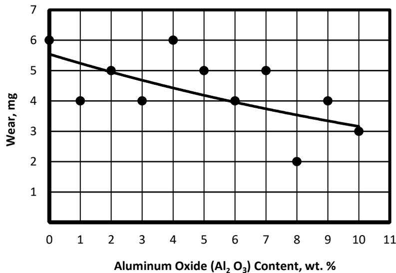
**Fig. 6** Effect of aluminum oxide nanopowder on wear of PE.
