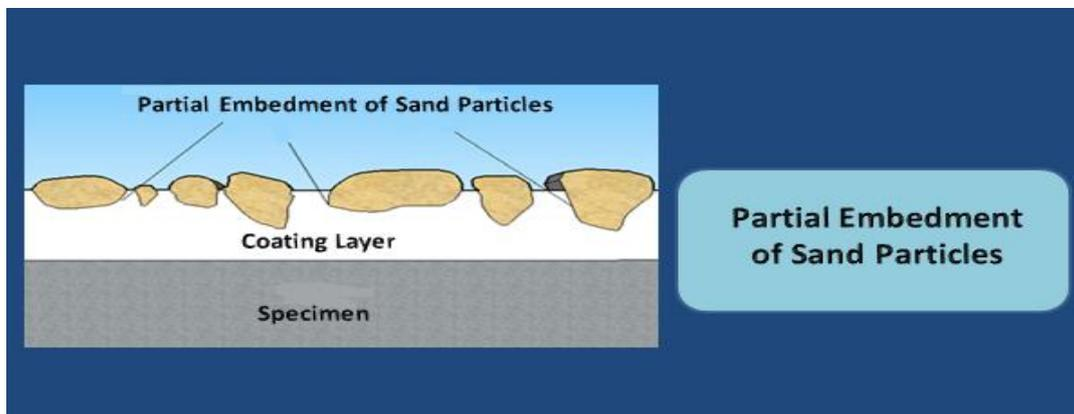
Fig. 11 Schematic illustration the embedment of sand particle.
