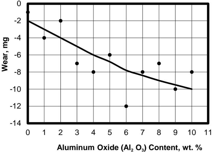
Fig. 23 Effect of aluminum oxide nanopowder on wear of PE filled by 10 wt. % oil content.
