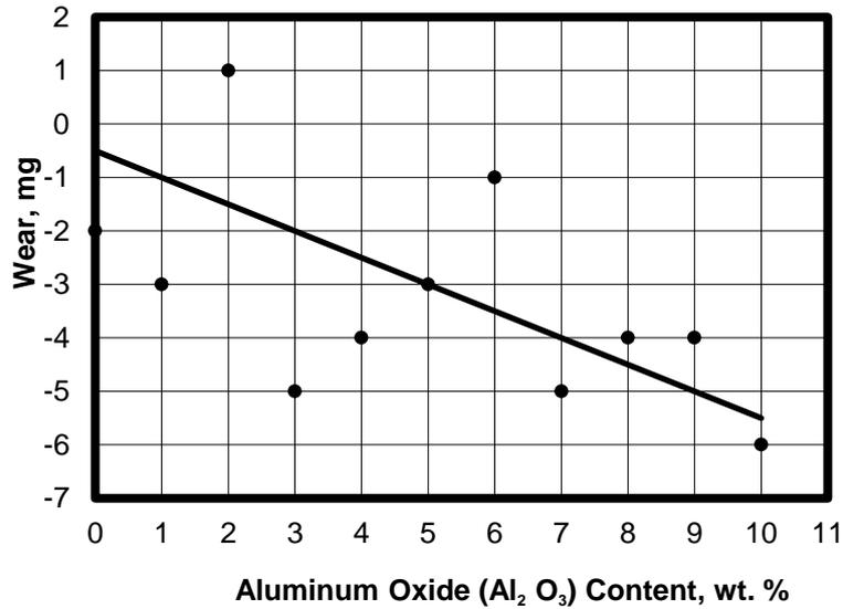
**Fig. 20** Effect of aluminum oxide nanopowder on wear of PE filled by 8 wt. % oil content.
