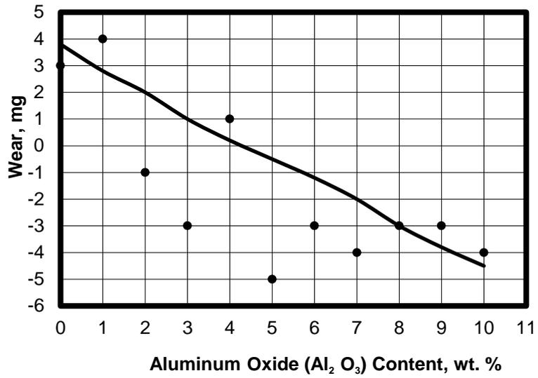
**Fig. 15** Effect of aluminum oxide nanopowder on wear of PE with 6wt. % oil content.
