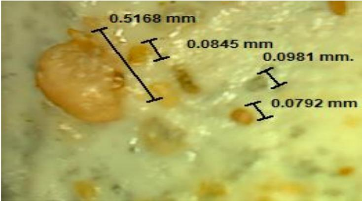
Fig. 22 Effect of sand particles size on embedment.
