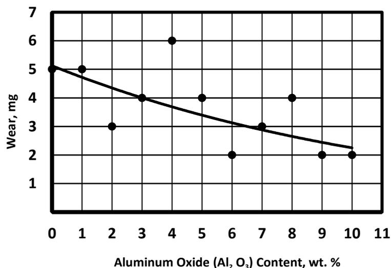
**Fig. 8** Effect of aluminum oxide nanopowder on wear of PE filled by 2 wt. % oil content.
