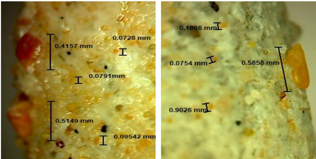
**Fig. 14. Effect of sand particles size on the embedment.**
