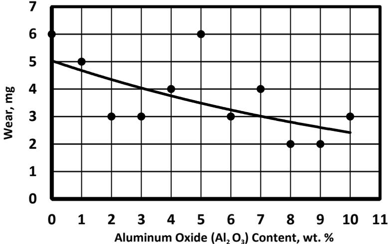
Fig. 9 Effect of aluminum oxide nanopowder on wear of PE filled by 3 wt. % oil content.
