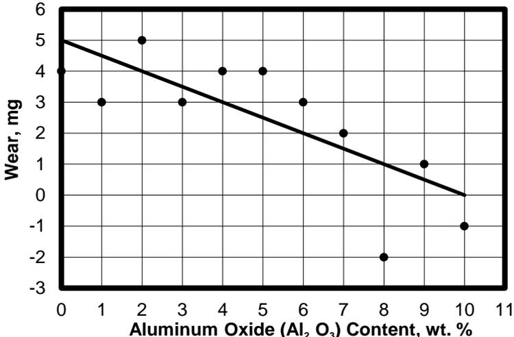
Fig. 10 Effect of aluminum oxide nanopowder on wear of PE filled by 4 wt. % oil content.
