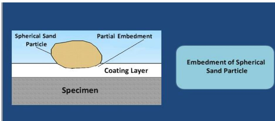
**Fig. 16.** Schematic illustration the embedment of spherical sand particle.
