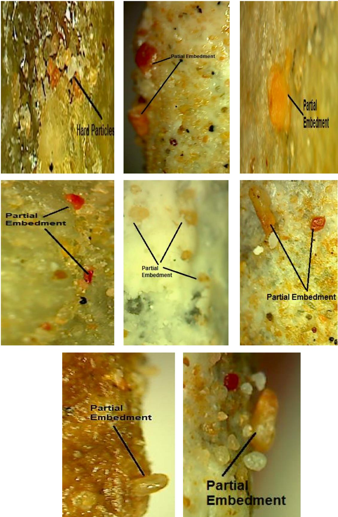
**Fig. 12 Photomicrographs of embedment of sand particles**
