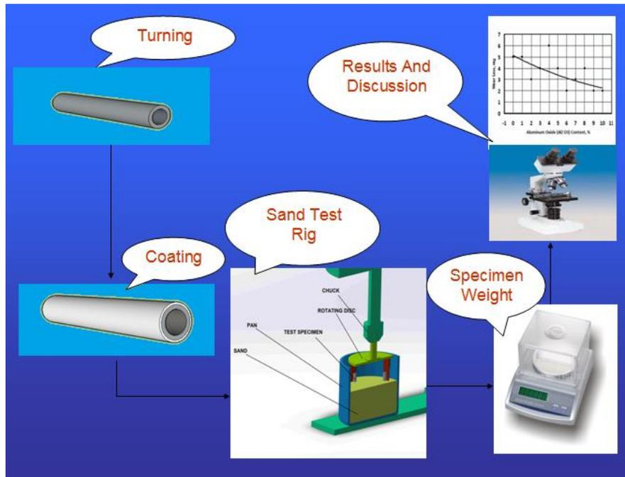
**Fig. 5** The sequence of the operations followed in the experimental work.
