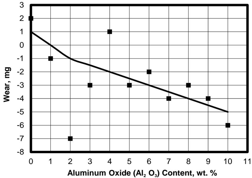
**Fig. 18 Effect of aluminum oxide nanopowder on wear of PE filled by 7 wt. % oil content.**
