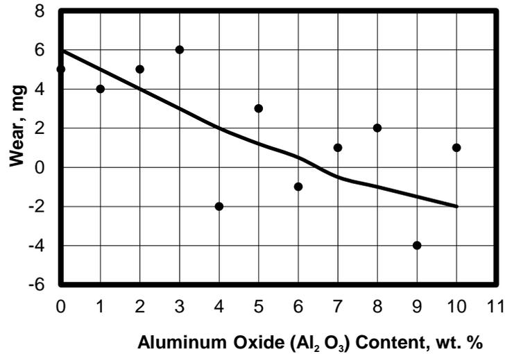
**Fig. 13 Effect of aluminum oxide nanopowder on wear of PE with 5 wt. % oil content.**
