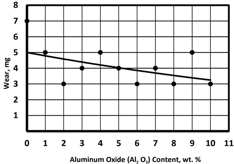
**Fig. 7** Effect of aluminum oxide nanopowder on wear of PE filled by 1wt. % oil content.
