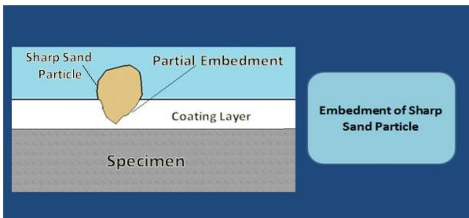
**Fig. 17.** Schematic illustration the embedment of sharp sand particle.
