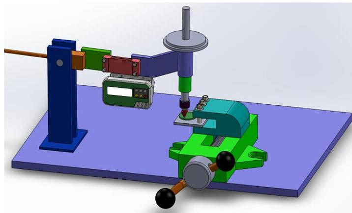
**Fig. 4 Arrangement of scratch test rig.**
