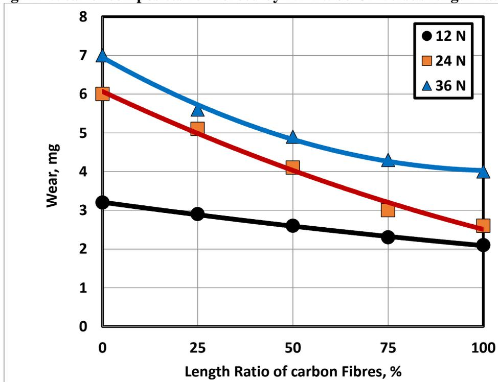
Fig. 12 Wear of composites reinforced by 4.5 wt. % CF versus length ratio.
