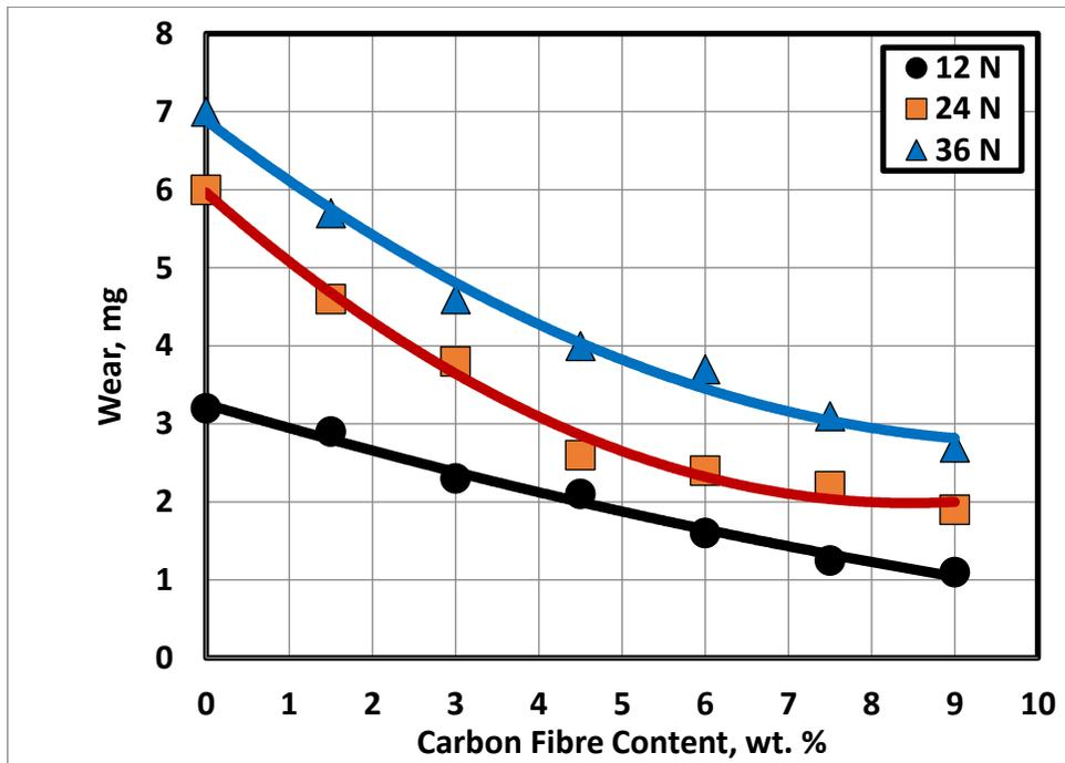
Fig. 10 Effect of CF content on adhesive wear of the tested composites.
