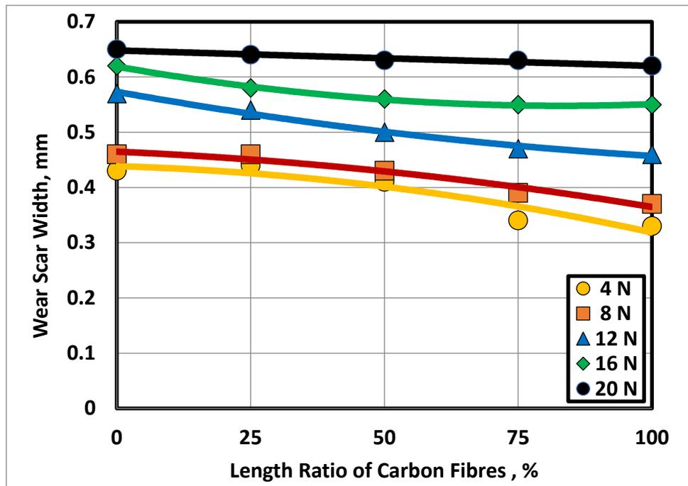
Fig. 21 Wear of the scratched composites reinforced by 7.5 wt. % CF versus length ratio.
