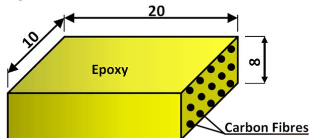
Fig. 1 Test specimens of scratch test.
