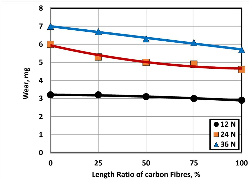
Fig. 11 Wear of composites reinforced by 1.5 wt. % CF versus length ratio.
