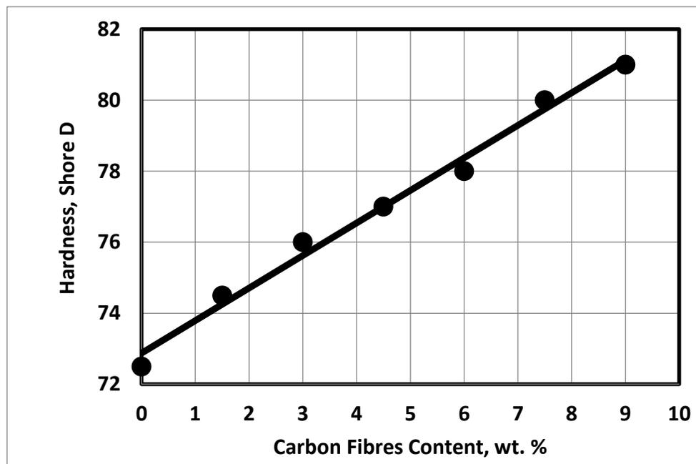
Fig. 5 Effect of CF content on hardness of the tested composites.
