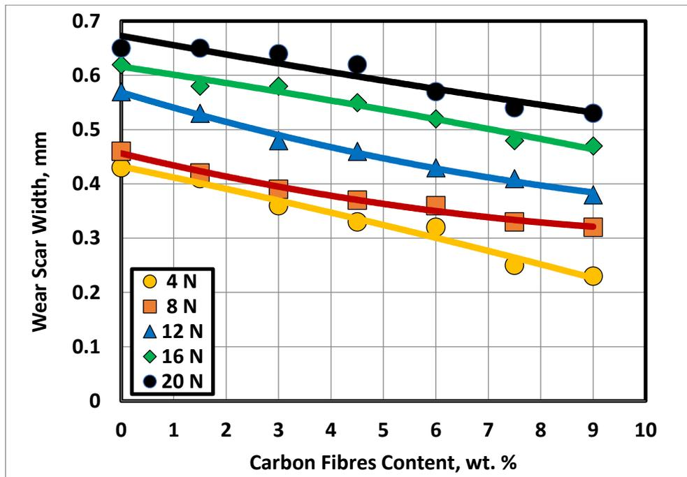
Fig. 18 Effect of CF content on wear of the scratched tested composites.
