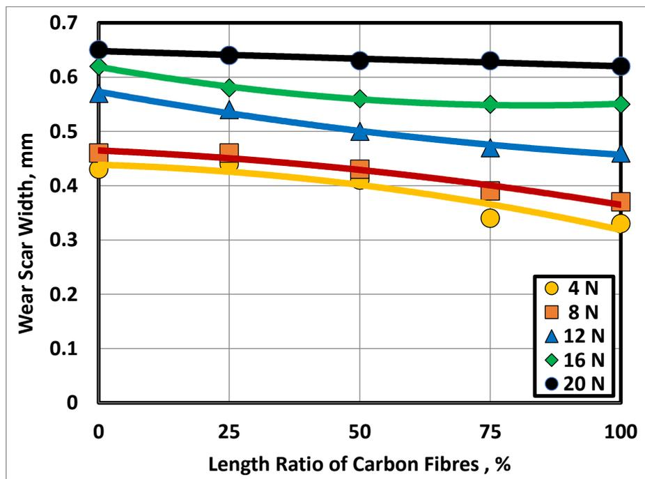
Fig. 20 Wear of the scratched composites reinforced by 4.5 wt. % CF versus length ratio.
