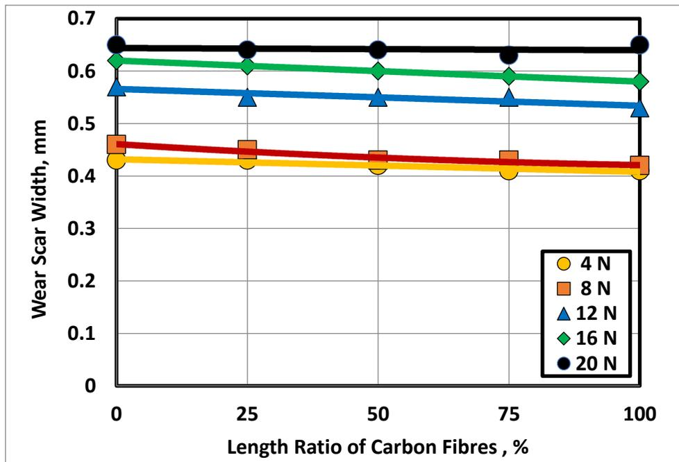
Fig. 19 Wear of the scratched composites reinforced by 1.5 wt. % CF versus length ratio.
