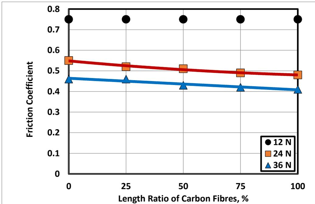
Fig. 7 Friction coefficient displayed by composites reinforced by 1.5 wt. % CF versus length ratio.
