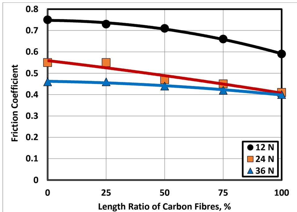
Fig. 8 Friction coefficient displayed by composites reinforced by 4.5 wt. % CF versus length ratio.
