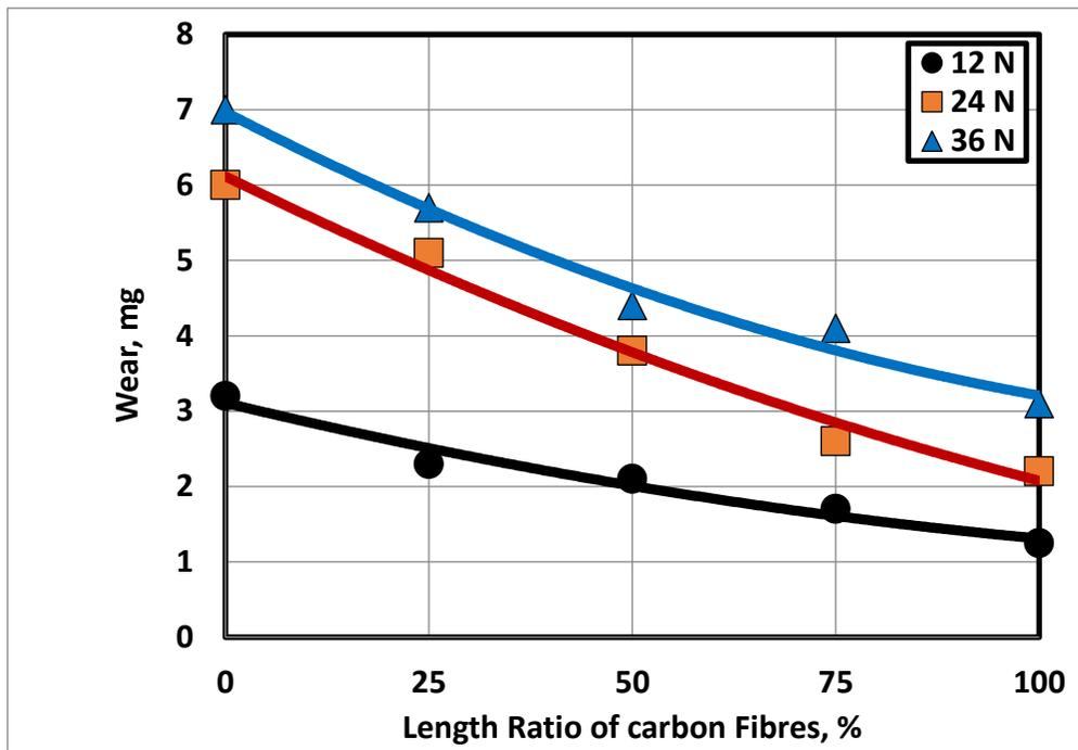
Fig. 13 Wear of composites reinforced by 7.5 wt. % CF versus length ratio.
