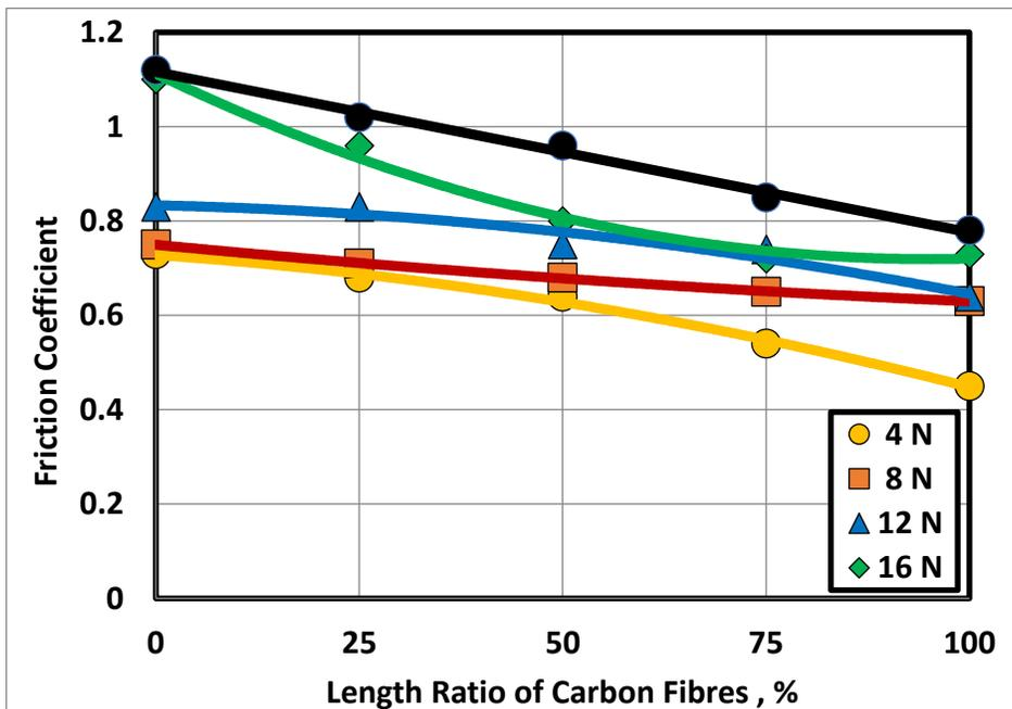
Fig. 16 Friction coefficient displayed by the scratched composites reinforced by 4.5 wt. % CF versus length ratio.
