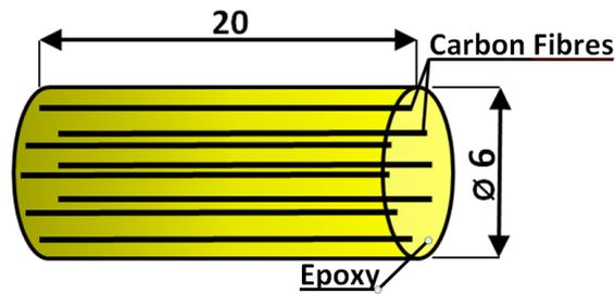
**Fig. 2 Test specimens of adhesion test.**
