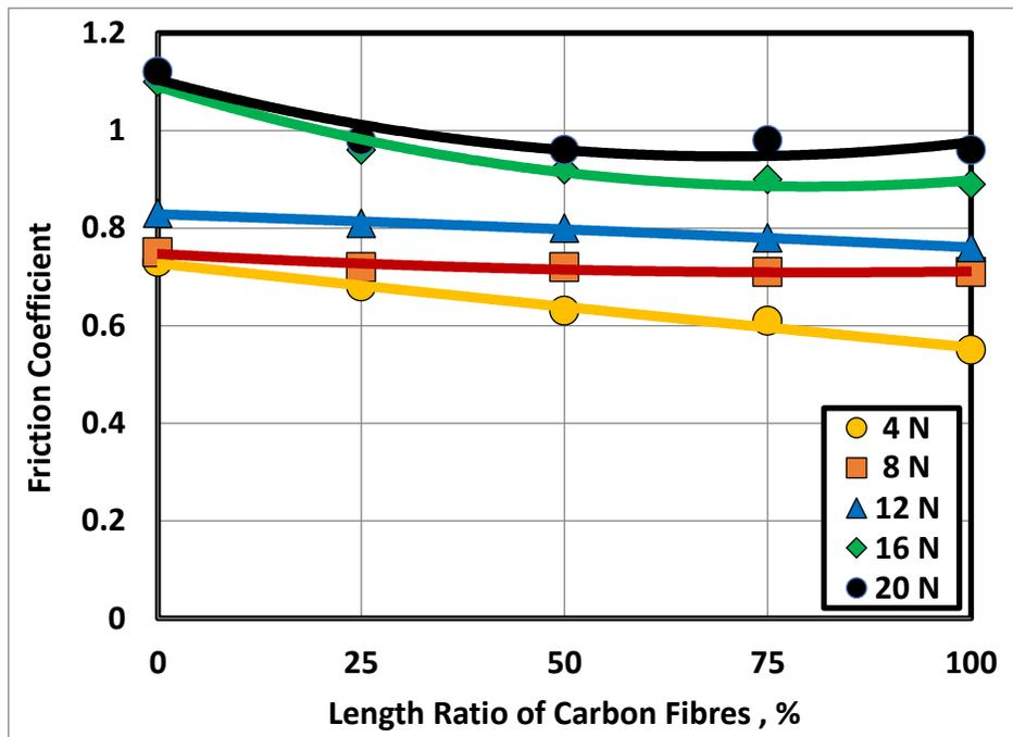
Fig. 15 Friction coefficient displayed by the scratched composites reinforced by 1.5 wt. % CF versus length ratio.
