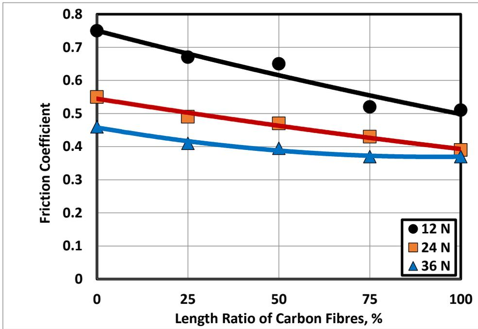
Fig. 9 Friction coefficient displayed by composites reinforced by 7.5 wt. % CF versus length ratio.
