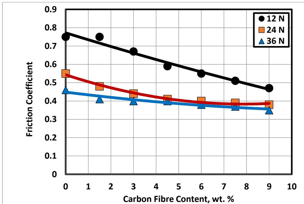
Fig. 6. Effect of CF content on friction coefficient of the tested composites.
