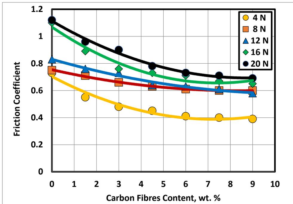
Fig. 14 Effect of CF content on friction coefficient of the scratched tested composites.
