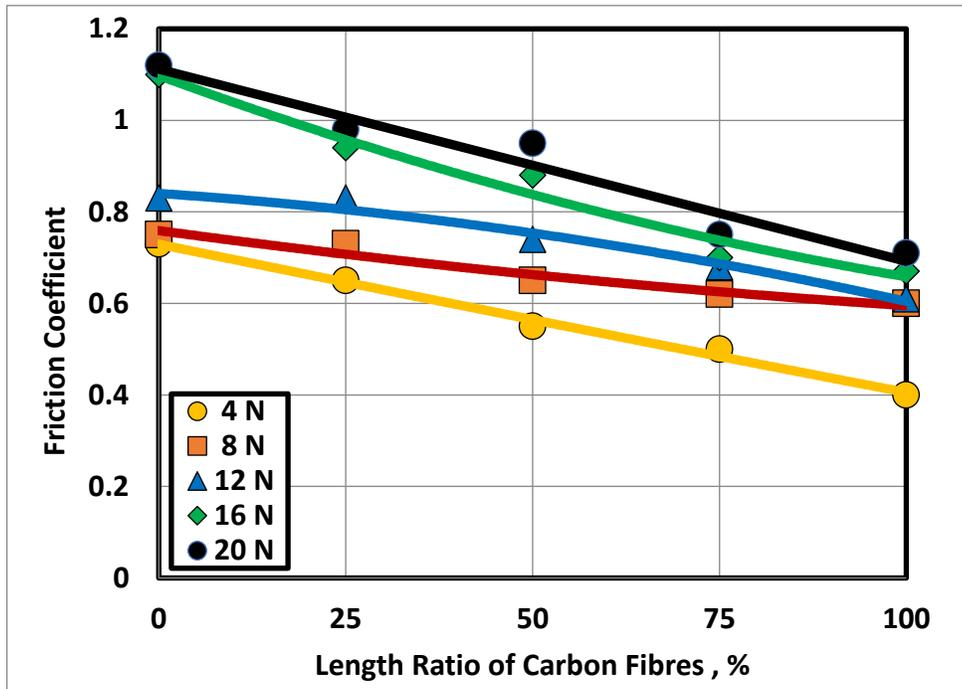
Fig. 17 Friction coefficient displayed by the scratched composites reinforced by 7.5 wt. % CF versus length ratio.
