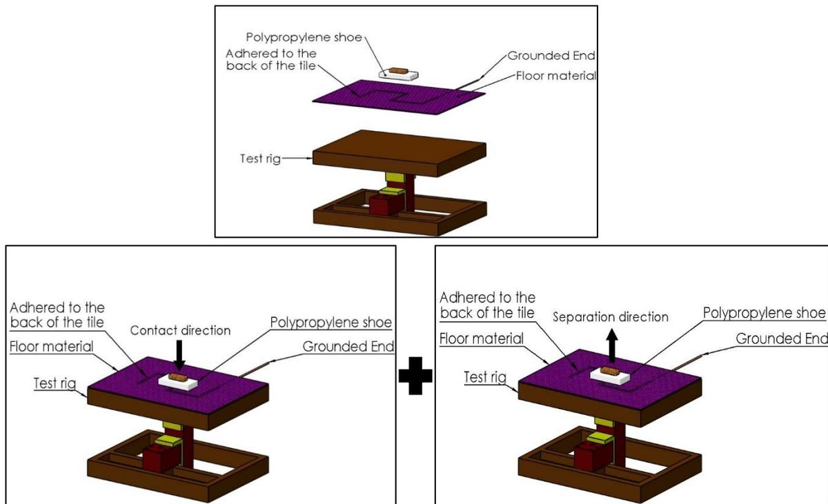
**Fig. 3 Arrangement of the experimental test.**
