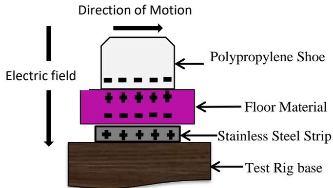
Fig. 5 Schematic illustration of ESC generated on ungrounded floor material.
