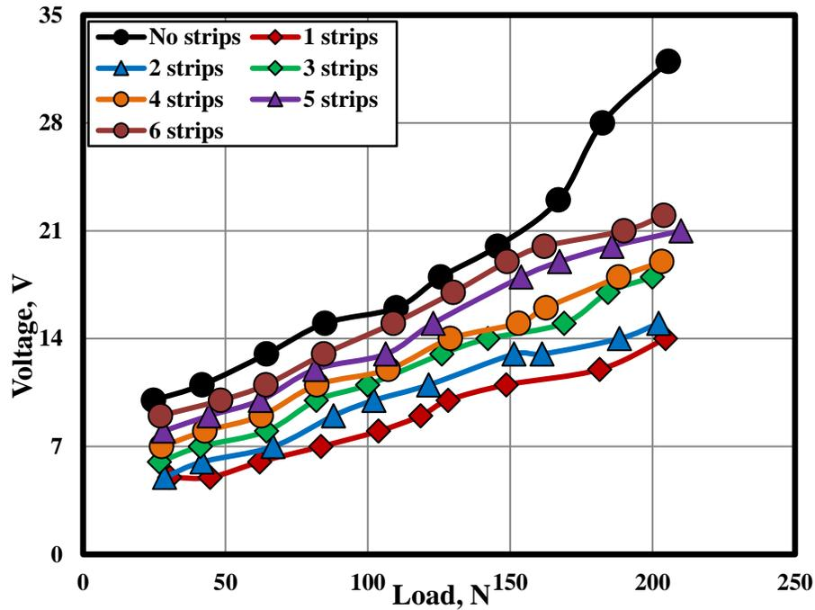
Fig. 8 Effect of number of strips on ESC on floor material (A) at chlorine wet condition and ungrounded.
