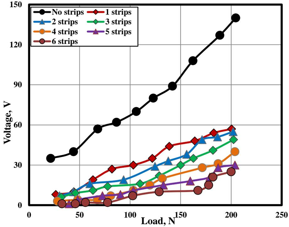
Fig. 6 Effect of number of strips on ESC on floor material (A) at grounded dry condition.
