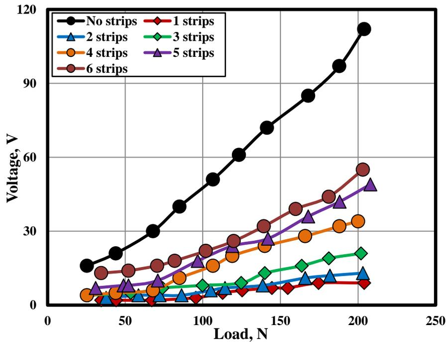
Fig. 7 Effect of number of strips on ESC on floor material (B) at ungrounded dry condition.
