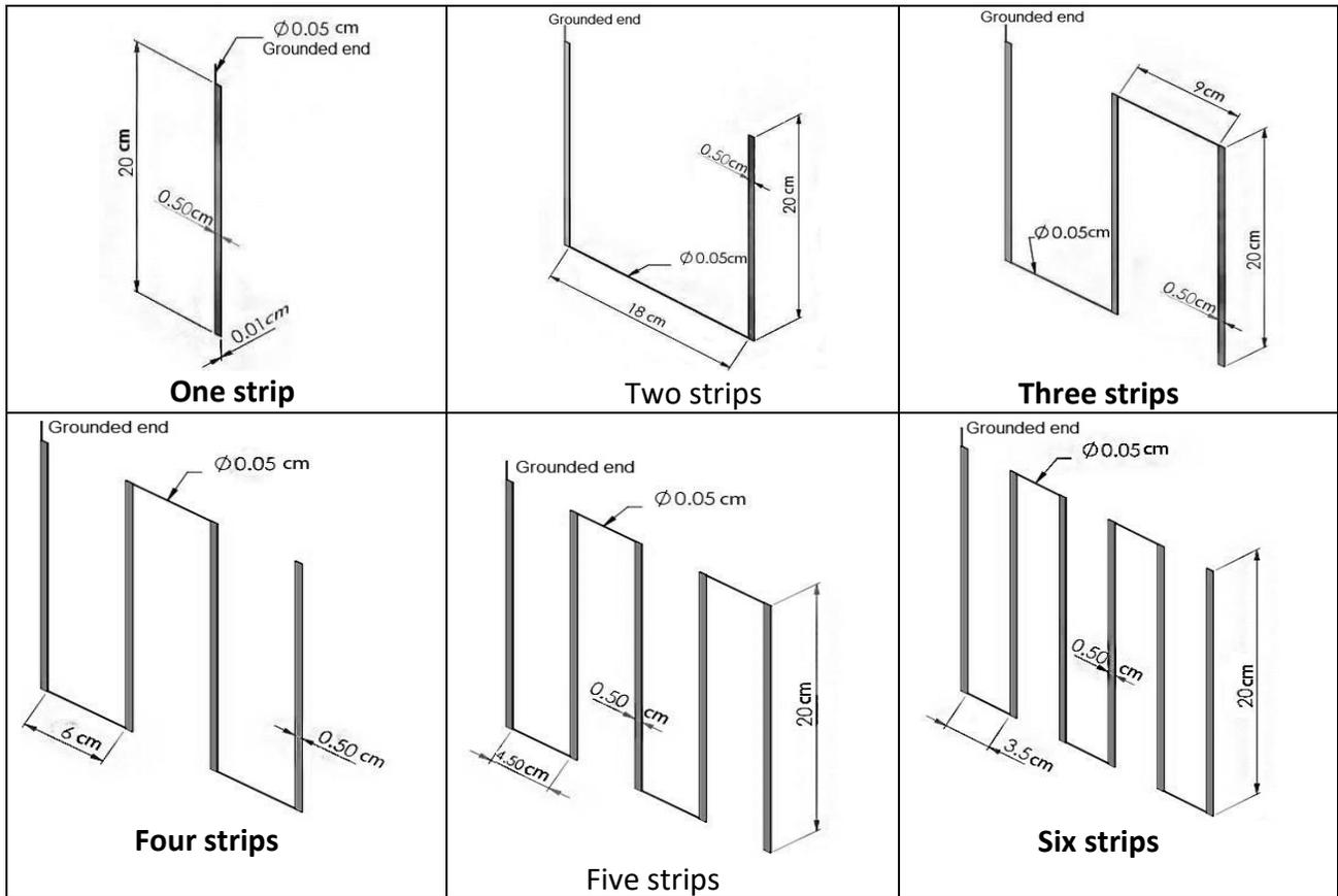
**Fig. 1 Distribution of the stainless steel strips.**
