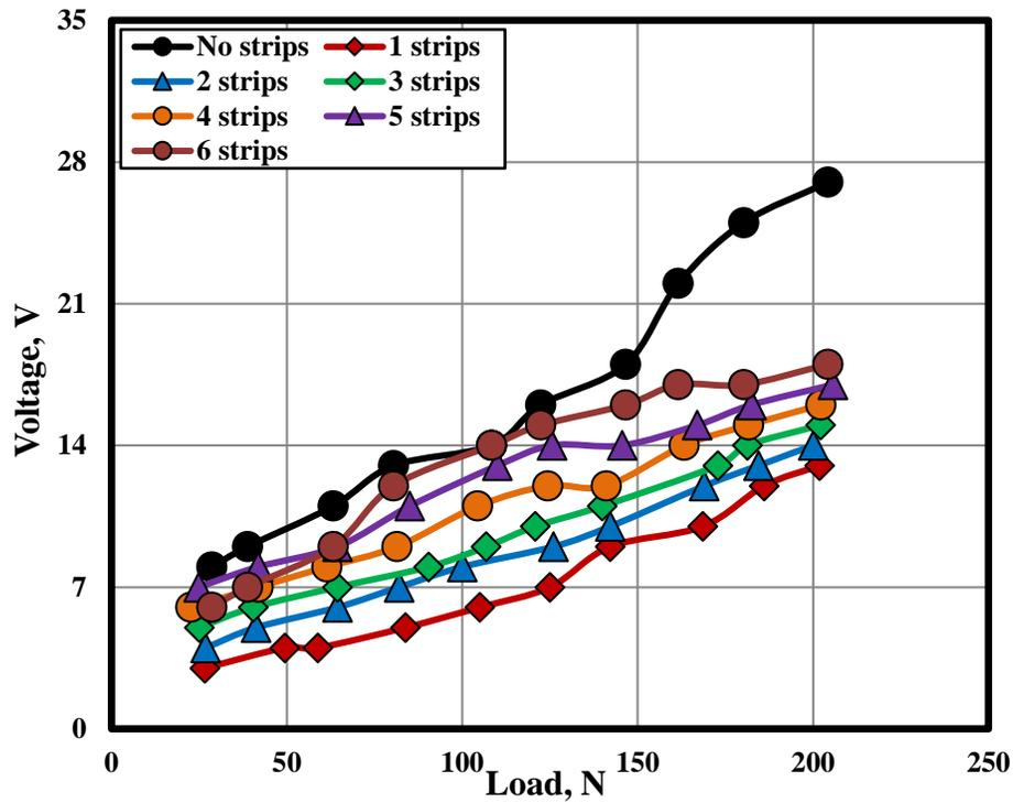
Fig. 10 Effect of number of strips on ESC on floor material (B) at ungrounded chlorine wet condition.
