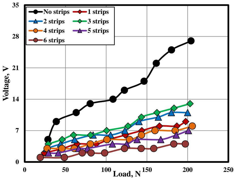
Fig. 11 Effect of number of strips on ESC on floor material (B) at grounded chlorine wet condition.
