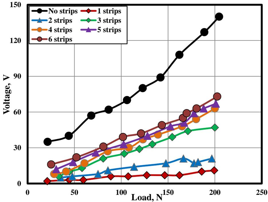
Fig. 4 Effect of number of strips on ESC on floor material (A) at ungrounded dry condition.
