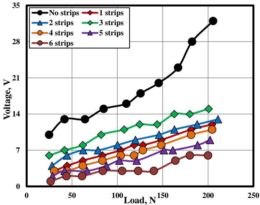
Fig. 9 Effect of number of strips on ESC on floor material (A) at chlorine wet condition and grounded.
