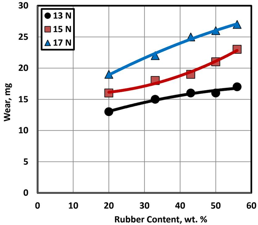
Fig. 7 Wear displayed by epoxy composites filled by rubber.
