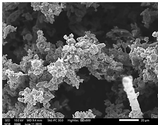
[c] CF/Epoxy composites filled by 10 wt. % corn oil.
