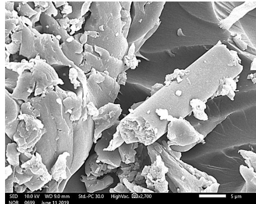
[f] CF/Epoxy composites filled by 10 wt. % paraffin oil.
