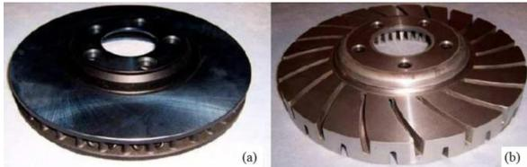
**Fig. 20** a) Brake disk (weight: 8.44 kg), manufactured from gray cast iron used in the sedan automobile, b) brake disc made of Al-SiC composite material (weight: 3.32 kg) specially designed for the same automobile [57].
