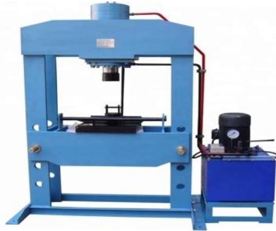
**Fig. 7** Uni Axial Hydraulic Press.
