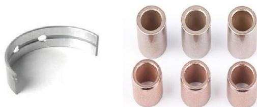
**Fig. 23** Crankshaft master bearings coated by FSM using a new alloy of Pb, Sn, Cu, and ZrO<sub>2</sub> powders.
