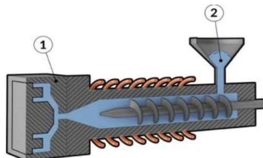
Fig. 11 Metal injection molding device.
