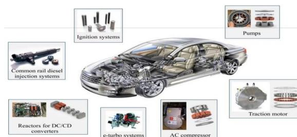
**Fig. 25** Main applications of SMC in automotive [72].
