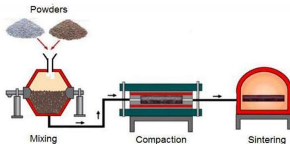
Fig. 9 The flow diagram in PSM production of parts.
