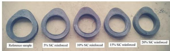
**Fig. 16** SiC reinforced Al-7075 matrix composite cams manufactured by PSM [53].
