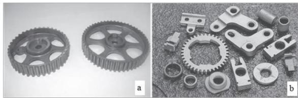
**Fig.19** Parts manufactured by PSM: a) Distribution pulleys, b) Fuel pump parts [56].
