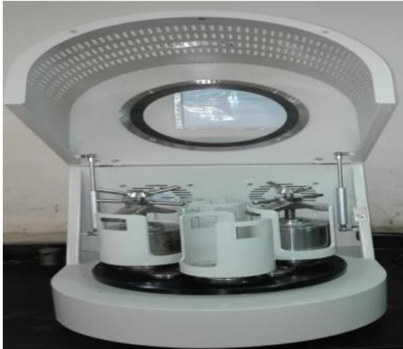
**Fig. 6** Four Vails Mechanical Mixer.
