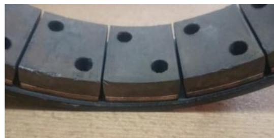
Fig. 27 Chain brake pads.
