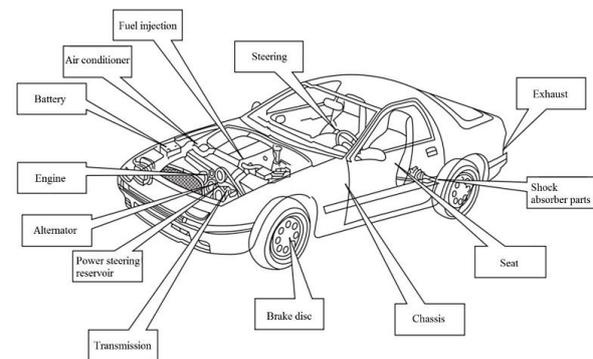
**Fig. 15** Different areas for PM applications in an automobile.
