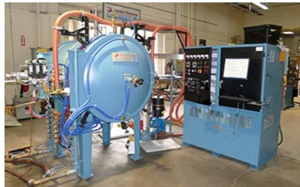
**Fig. 8** Vacuum Sintering Furnace
