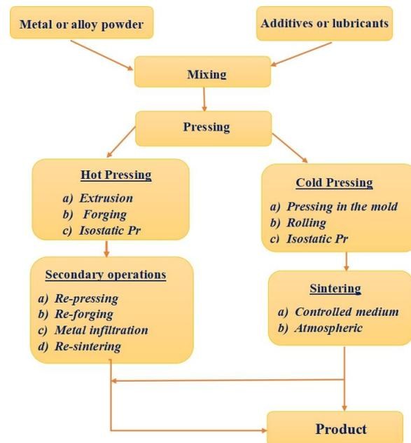
Fig. 5 Flow chart of the conventional PM process.
