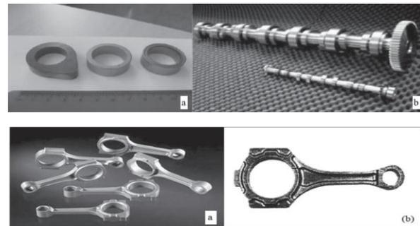
**Fig. 17** Composite motor components produced by PSM: a) Cam and intermediate rings, b) Camshaft [54].
