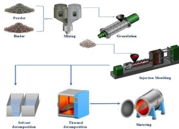
Fig. 10 Powder injection molding steps [19].
