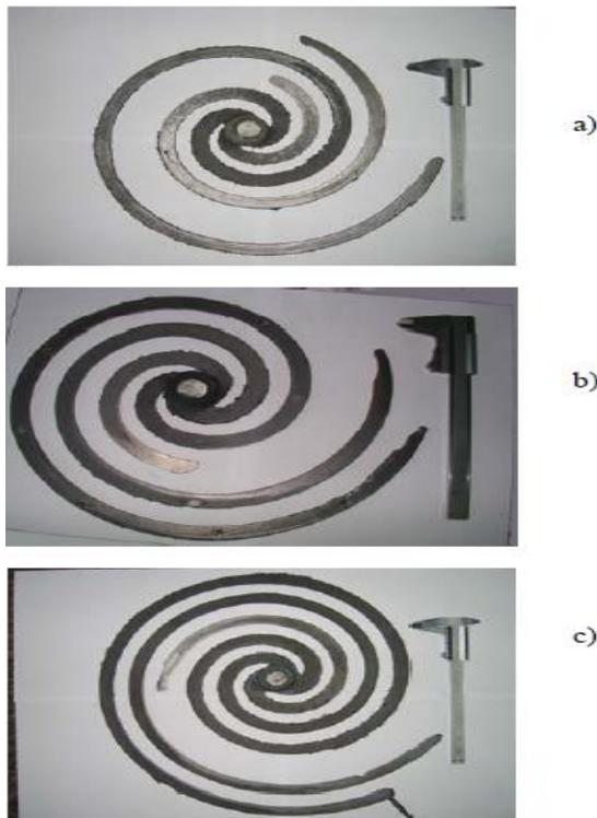
**Fig. 3** Castability of spirals of 3mm wall thickness poured into mold with different molding materials: classical a), SHMS b) and SHMS with LDASC c) [12].
