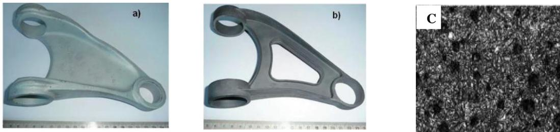
**Fig. 9** Control arms made from: (a) forged Al- alloy (weight 585 g), (b) TWDCI (weight 480 g) and (c) microstructure after heat treatment [2].
