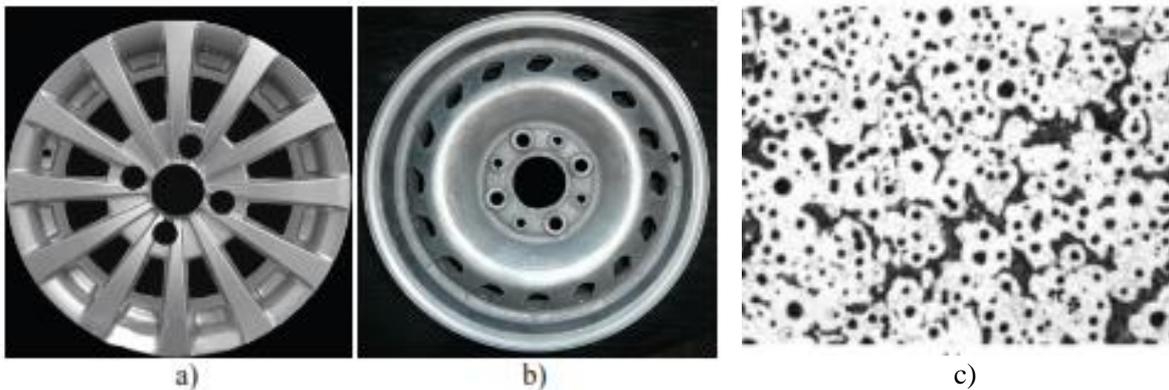
**Fig. 11** Wheel rim produced from Al-Si7Mg alloy – a), wheel rim produced from DI – b) and microstructure of thin wall ductile iron in wheel rim (2mm) - c) [8].
