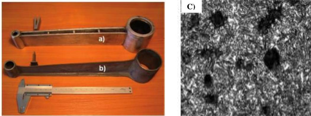
**Fig. 10** Cantilevers made from: (a) Al- alloy (weight 580 g), (b) TWADI (weight 380g) and (c) microstructure after heat treatment [2].
