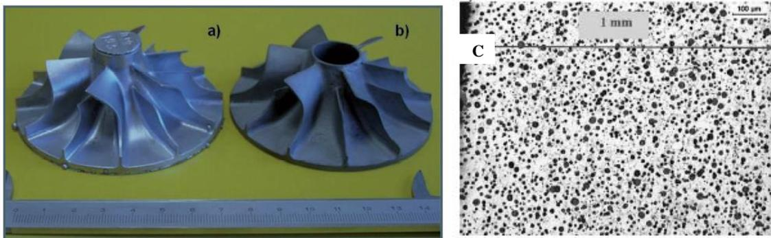
**Fig. 8** Rotors: (a) aluminum alloy, (b) TWDCI and (c) structure of rotor vane with 1.0 mm wall thickness [2].
