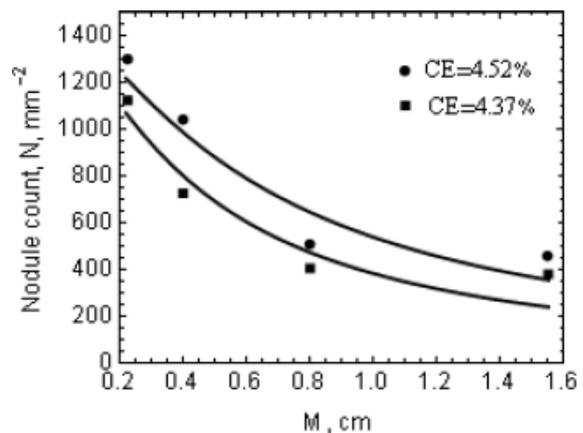
**Fig. 4** Nodule count for different values of carbon equivalent (CE),  $CE = C + 0.33Si$  [8].
