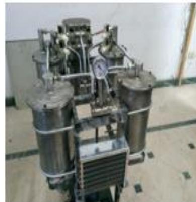
Fig.4: Photo of adsorption desalination unit
