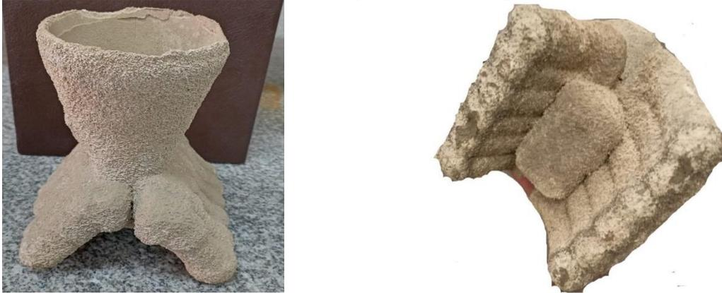
**Fig. 1. Investment mold containing six tensile and impact specimens**
