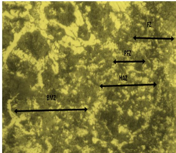
**Fig. 6** Microstructure of partial fusion zone, X 1000.
