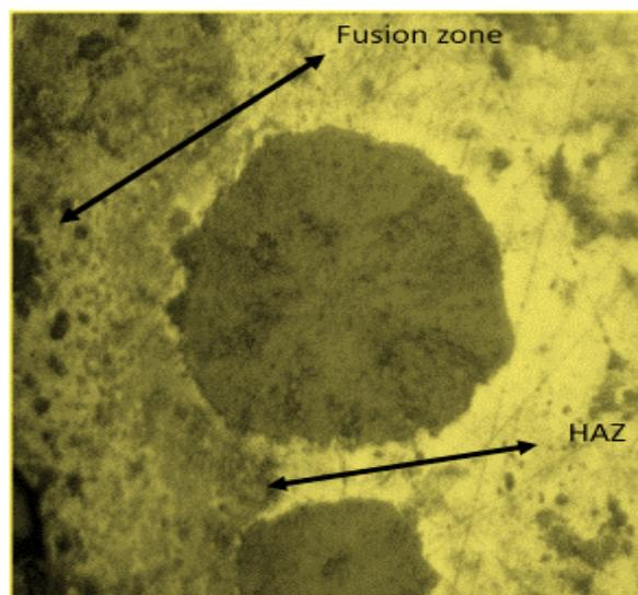
**Fig. 5** Microstructure of the fusion zone of heat-affected zone X1000.
