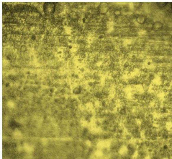
**Fig. 7** Microstructure of the austenite transformation zone, X1000.
