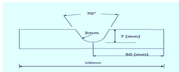
**Fig. 1** Configuration and dimension of Arc welding specimen.
