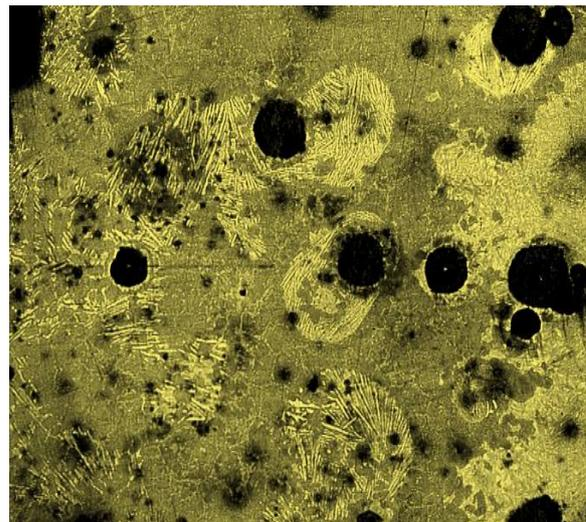
**Fig. 8** Microstructure of repeated transformation zone, X1000.
