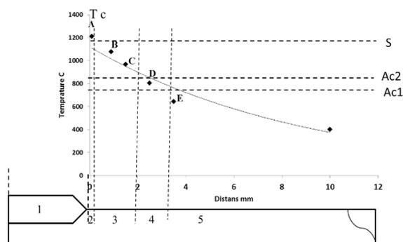
**Fig. 4** The highest temperature distribution across welding joint.
