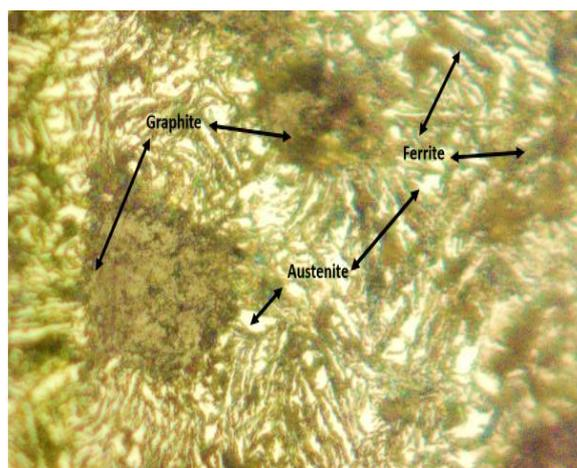
**Fig. 2** microstructure of base metal (Ausferrite structure) X1000.
