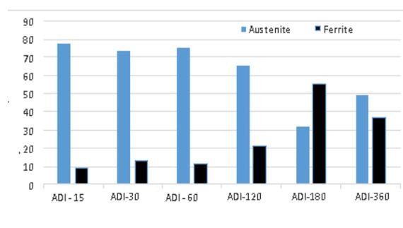
**Fig. 3** Volume fraction percentage (Austenite and Ferrite) of ADI alloys under study.
