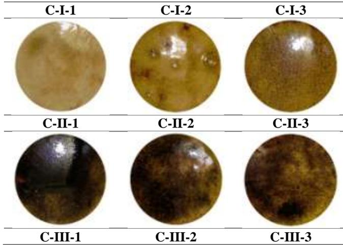
**Fig. 5** Digital photographs of glaze samples of different types of clay.
