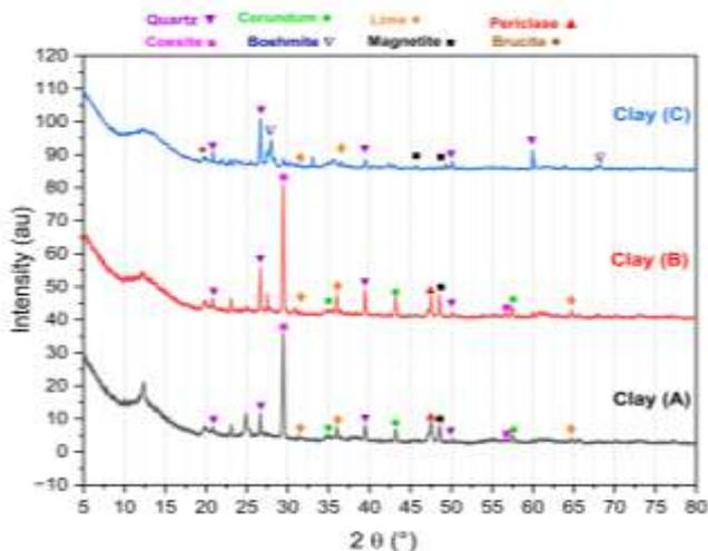
**Fig. 4.** XRD pattern for different types of clay used in this study show the crystal structure of each materials composition.
