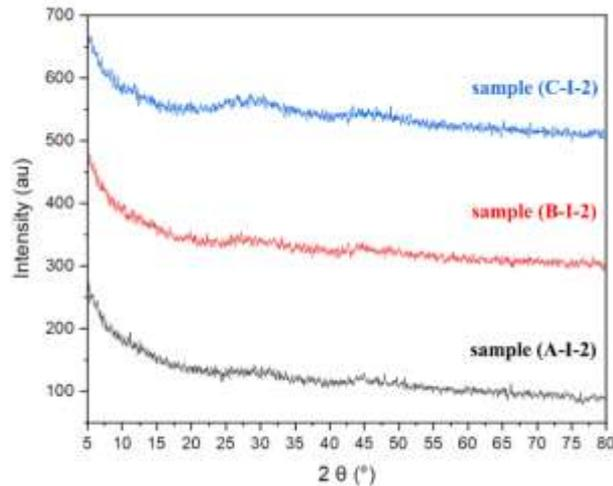
**Fig. 6.** XRD pattern of samples A-I-2, B-I-2, and C-I-2 cristobalite.
