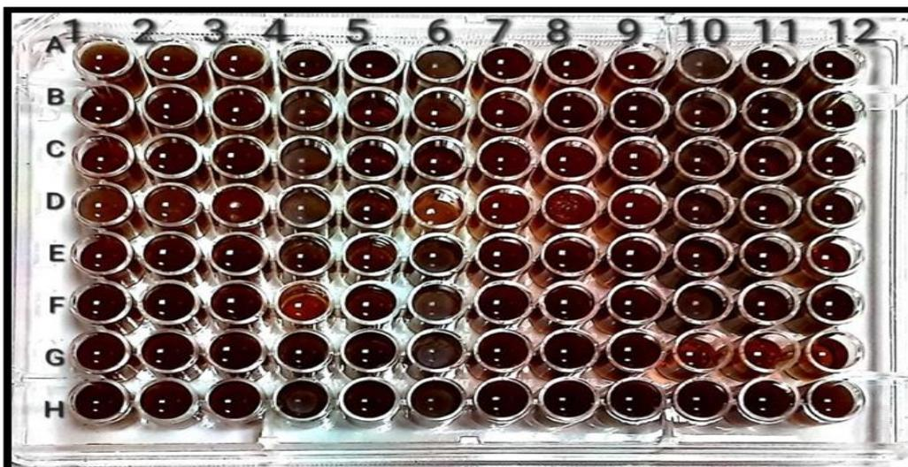
Row A: showed two isolates, columns 1, 2, and 3 contained isolate no.1 without AgNPs, and columns 4,5,6 contained the same isolate no.1 in addition to AgNPs, and isolate no.2 in columns (7,8,9), and so on till row H (column 6). Row H (columns 7, 8, 9, 10, 11, 12) contained tryptone soya broth only.
